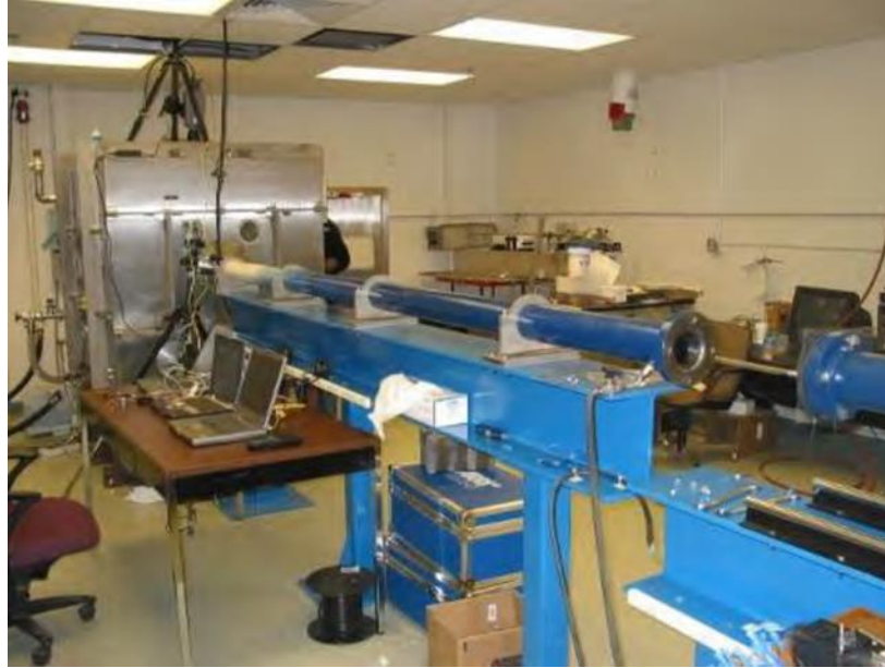
Figure 110. Large vacuum gas gun
