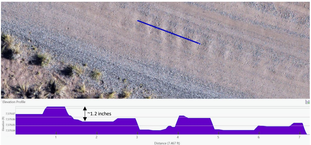
Figure 7. Example measurement of washboarding depth
