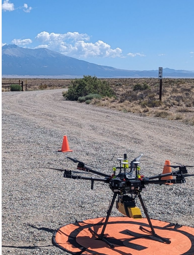
Figure 3. DJI Matrice 600 Pro with YellowScan VX20-100 lidar
