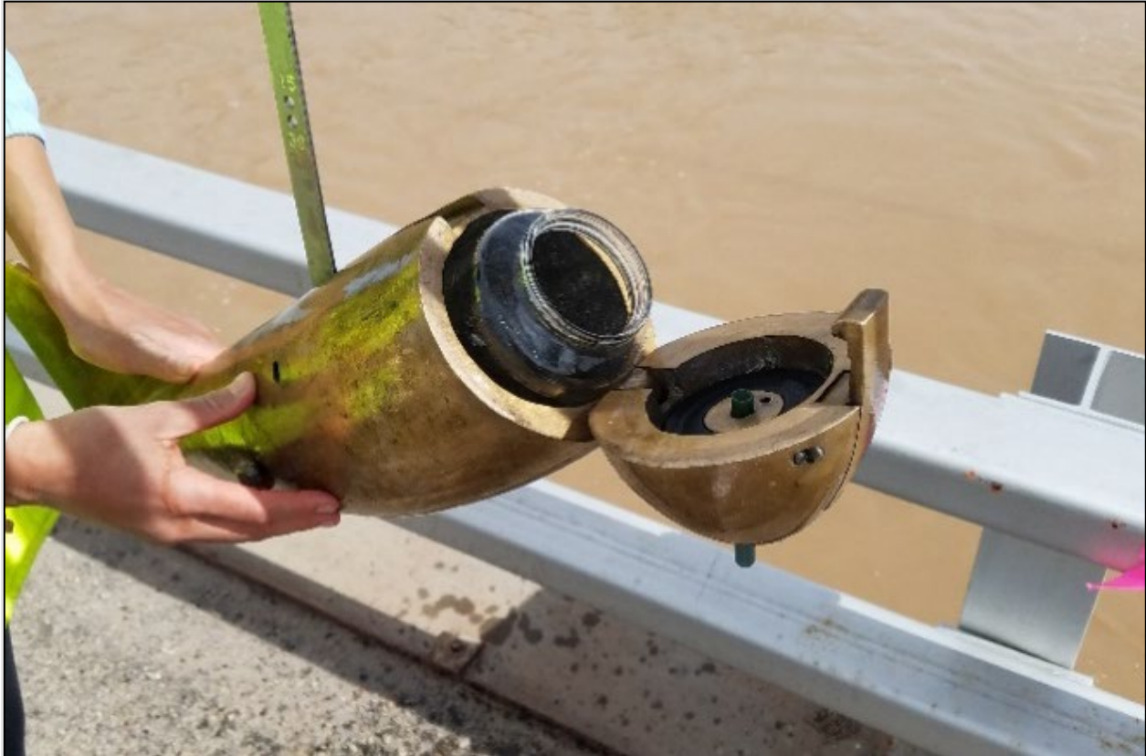
Figure 7.4. D-74 suspended sediment sampler open and ready to empty sample of water-sediment mixture in the Rio Grande at the New Mexico 147 bridge. Image used by permission of Tetra Tech, Inc.
