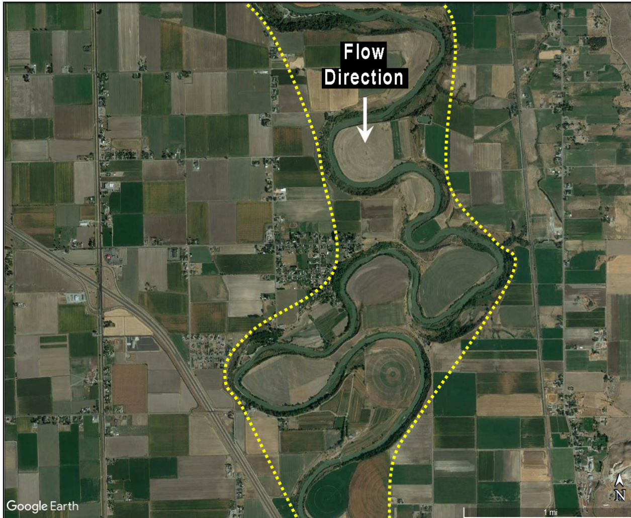
Figure 6.17. Dotted lines illustrate a potential meander belt width based on 2018 aerial imagery for a reach of the Bear River, UT.
