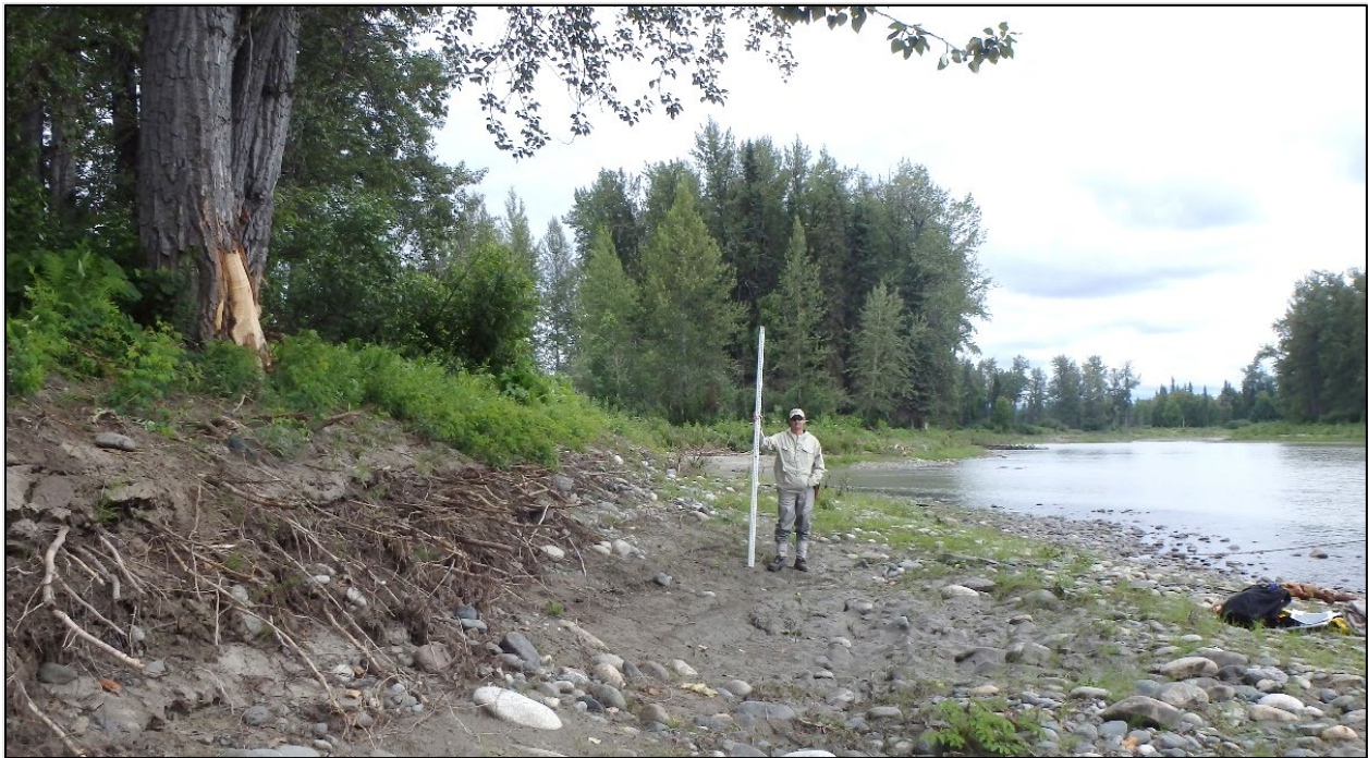
Figure 8.6. Photograph demonstrating the effects of ice abrasion. Image used by permission of Tetra Tech, Inc.
