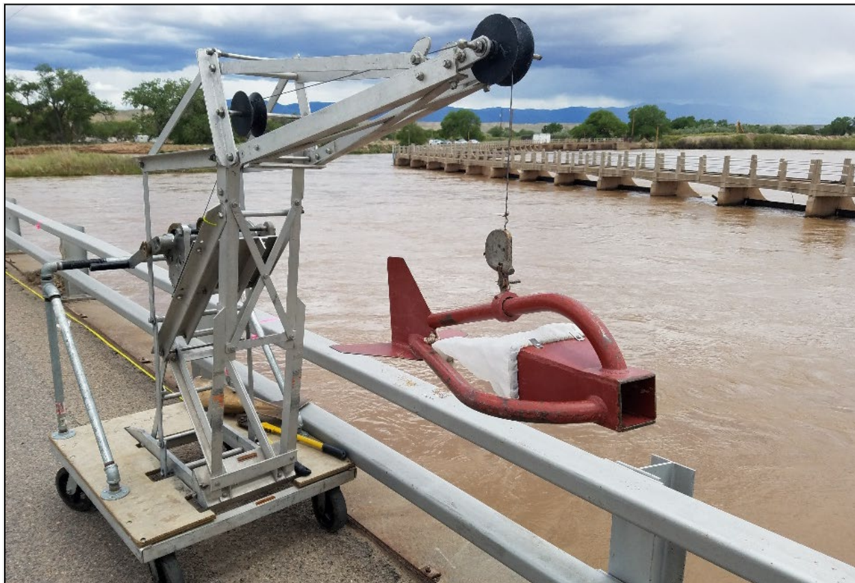
Figure 7.5. Helley-Smith bed load sampler used to measure near-bed sediment load in the Rio Grande at the New Mexico Highway 147 bridge. Image used by permission of Tetra Tech, Inc.
