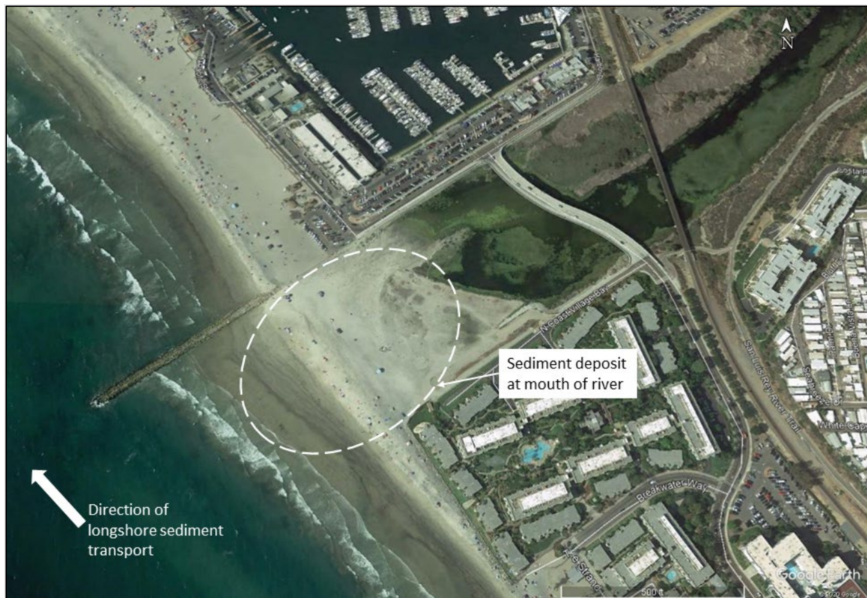
Figure 8.23 Effect of longshore sediment transport at the mouth of the San Luis Rey River, California.
