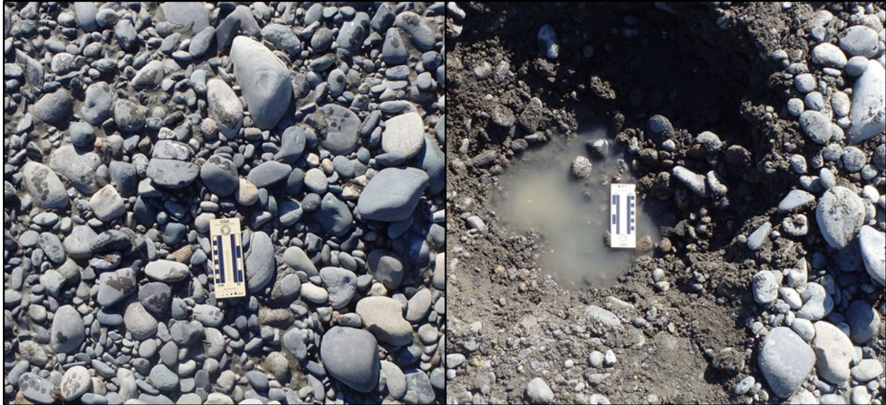
Figure 2.7. Example of armor layer with minimal sand present and substantial sand exposed when the armor is removed. Image used by permission of Tetra Tech, Inc.
