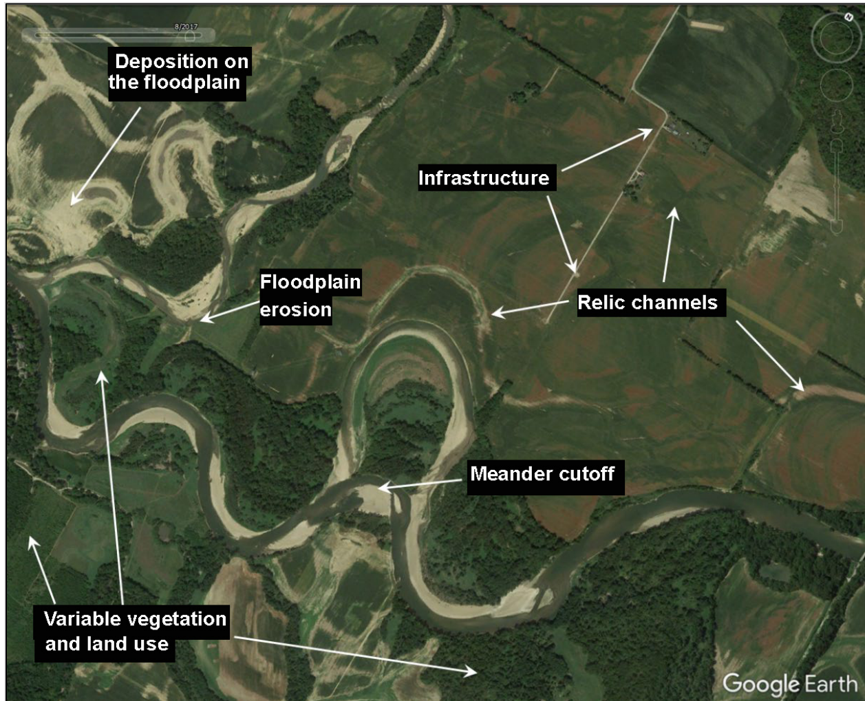
Figure 2.25. Complex connected floodplain with bend cutoff, relic channels, erosion and deposition, infrastructure, and highly variable vegetation cover and land-use.
