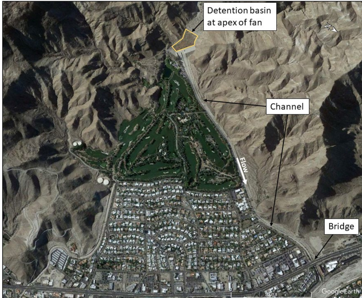
Figure 8.19 Aerial view of Magnesia Spring Canyon alluvial fan in Rancho Mirage, California.
