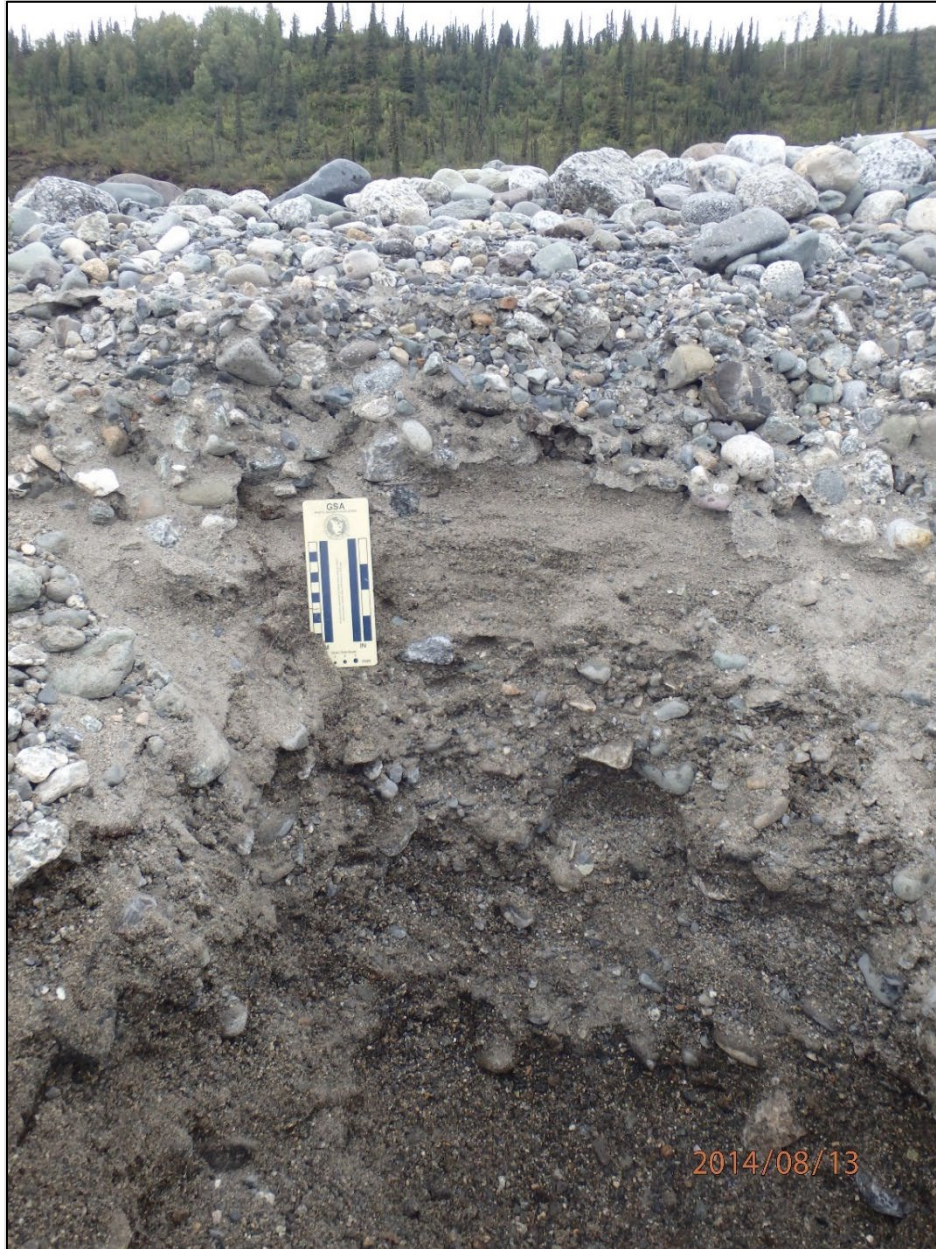
Figure 6.10. Sediment sample hole demonstrating the coarse armor layer and several gravel and sand layers below. Image used by permission of Tetra Tech, Inc.
