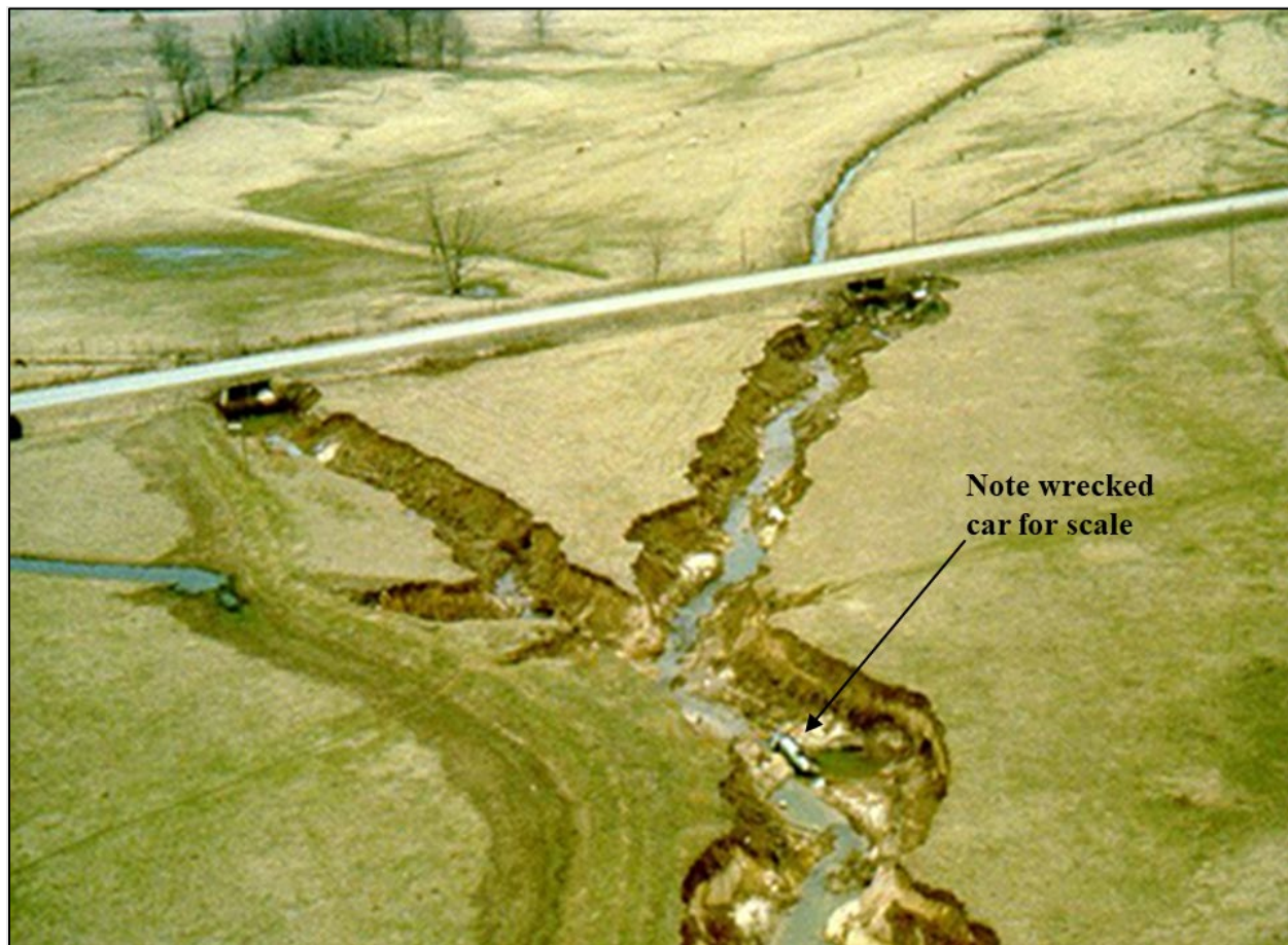
Figure 6.37. Example of the consequences of vertical instability at Crowder Creek, Leake County, Mississippi. Image used by permission of D. Biedenbarn (© 1985).
