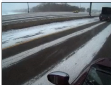
Snow may be cleared from wheel tracks but still cover lane markings, impeding the lane-finding function in AVs.
