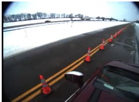
Figure 38. Tests with traffic cones to evaluate what density of cones prevents the Mobileye lane boundary detection system from working.
