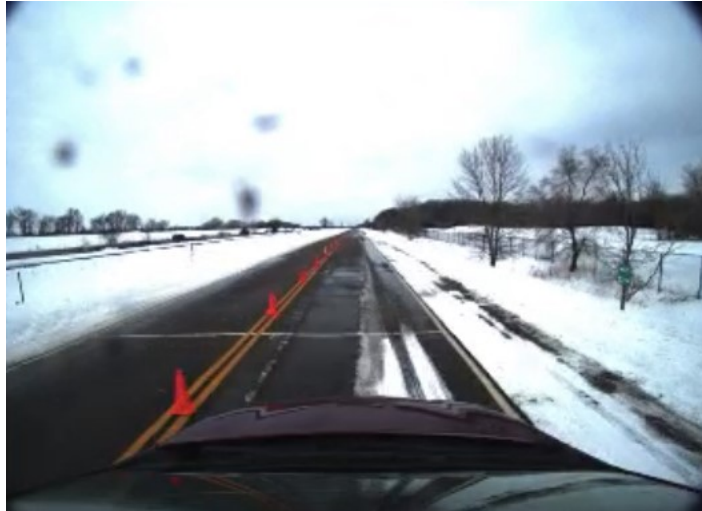
Figure 27. Cone test setup on top of lane lines with 6ft spacing.
