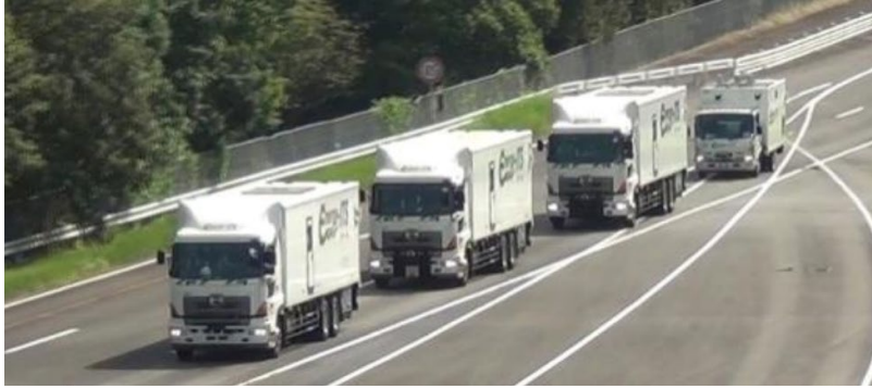
Figure 4. Photos. Configuration of automated platoon of 3 heavy trucks and a light truck.
