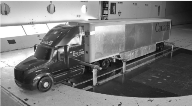
Figure 6. Photo. Truck platoon model in wind tunnel. Source: McAuliffe and Ahmadi-Baloutaki, 2018
