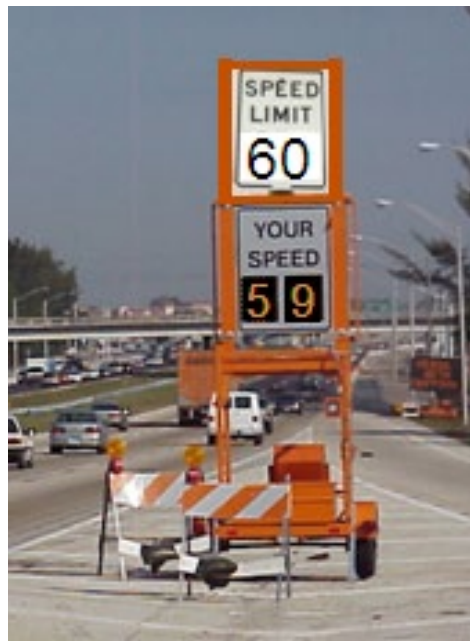
Figure 6. Photo. Speed displays in work zone.
