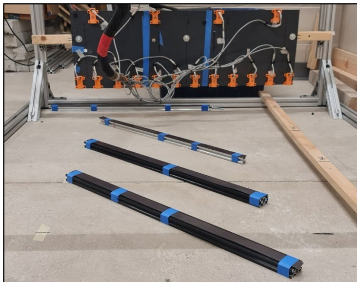
Figure 23. Photo. Experimental setup for EM-sensing strips placed at an angle to sensor arrays.
