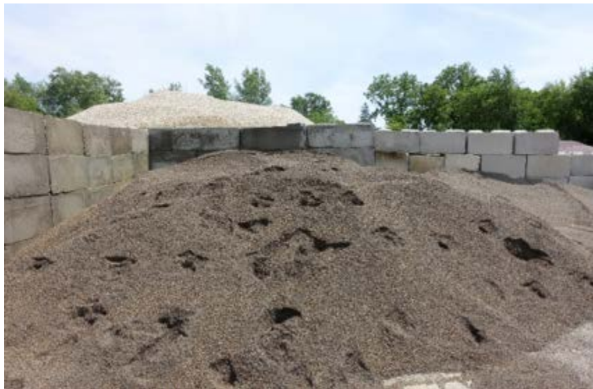
Figure 2.2: Lightweight Aggregate Stockpile for MN-IC-LC-HPC-2
