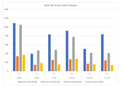
Figure 15. Comparison of HIC15 results for the Volkswagen Arteon with its hood in the normal state and fully deployed state at 40 kph and 26 kph headform impact speeds
