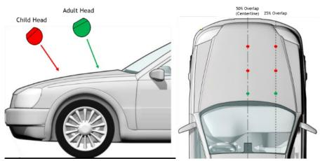
Figure 6. Crashworthiness pedestrian headform impact setup and impact locations
