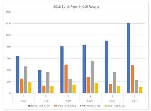
Figure 14. Comparison of HIC15 results for the Buick Regal with its hood in the normal state and fully deployed state at 40 kph and 26 kph headform impact speeds
