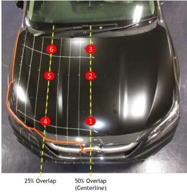
Figure 10. 2020 Subaru Outback pedestrian headform impact locations
