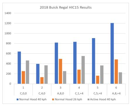
Figure 16. Reduction of HIC15 values for the Buick Regal due to a reduction of impact speed versus the presence of an active hood
