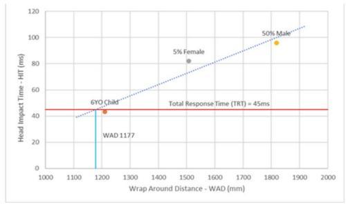
Figure 8. Head impact time (HIT) versus wrap around distance (WAD) and the relationship with the active hood total response time (TRT)
