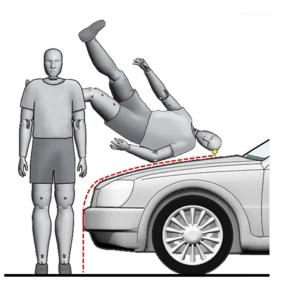
Figure 7. Wrap around distance (WAD) for a given stature shown by the red dotted line
