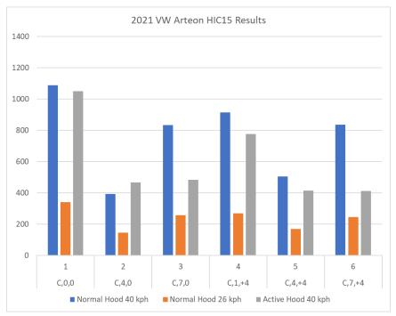
Figure 17. Reduction of HIC15 values for the Volkswagen Arteon due to a reduction of impact speed versus the presence of an active hood
