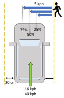
Figure 5. PAEB test scenarios S1a (25%), S1b (50%), and S1c (75%)
