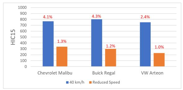
Figure 13. Average HIC15 values at 40 kph and reduced speeds for each of the vehicles tested (probabilities of death are shown in red)
