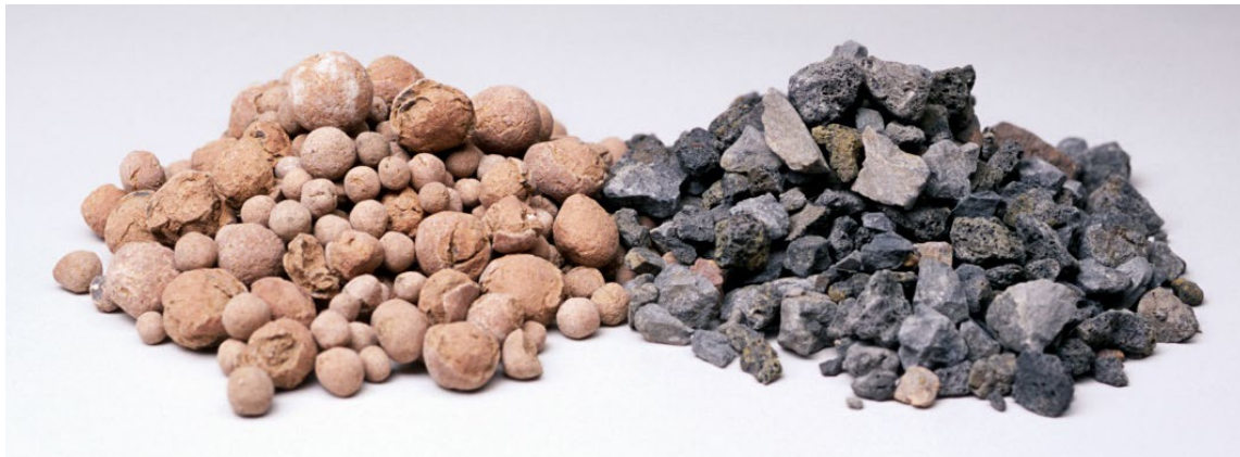
Figure 2. Photo. Lightweight aggregates from two different sources: uncrushed and crushed.
