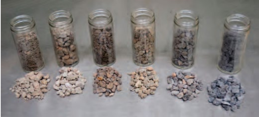
Figure 3. Photo. Different types of lightweight aggregates tested by Cousins et al. (2013). From left to right: Clay1, Shale1, Shale2, Clay2, Shale3, and Slate1. All of these lightweight aggregates are crushed.
