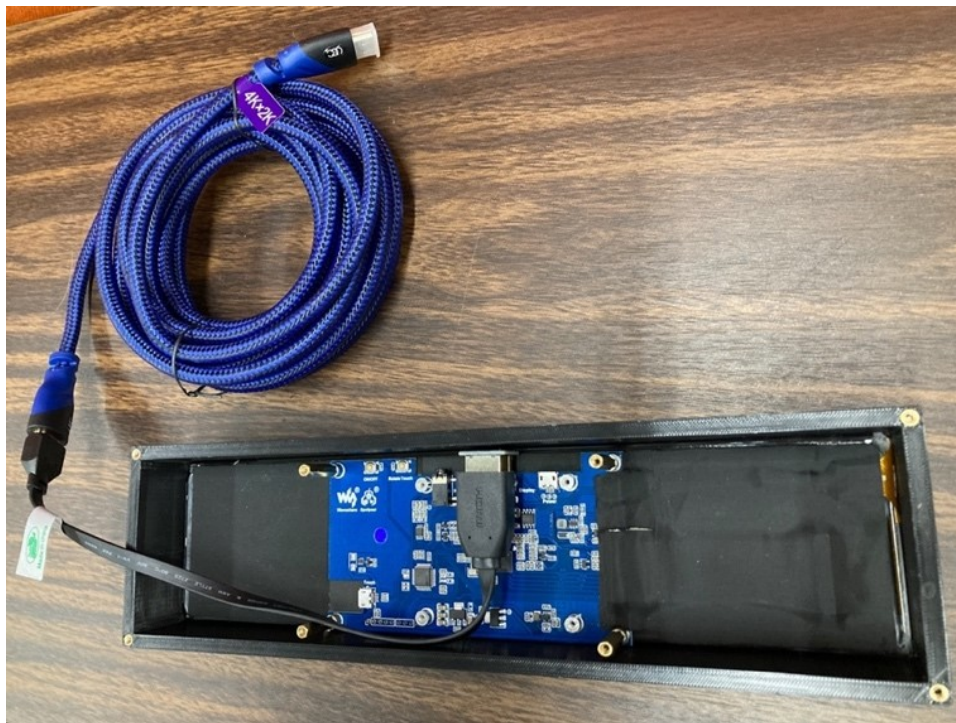
Figure 6.4 Display electronics in enclosure without backplate
