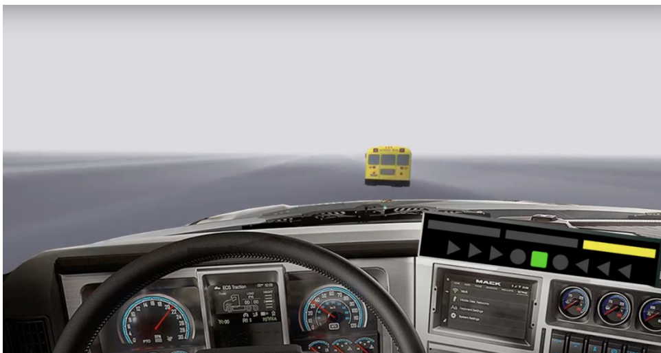
Figure B-2 Three screen shots of Flashing Location Bar indicator for center, left, and right hazard
