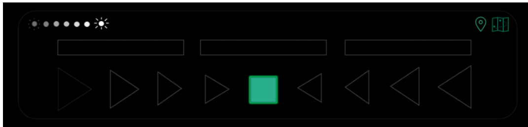
Figure 8.1 Screenshot the five brightness levels (see top left corner) and of GPS and Mapping icons indicating GPS and mapping are available (the icons are in the upper right corner)
