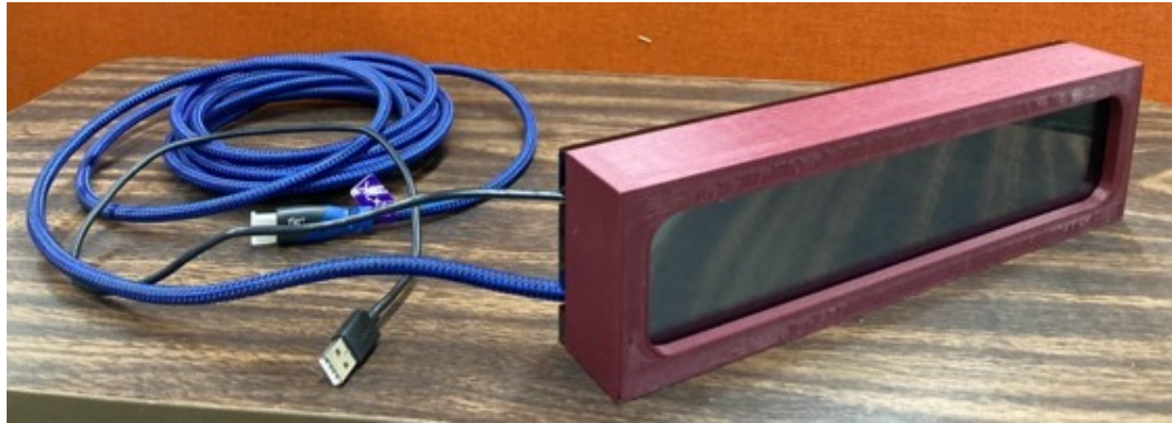
Figure 6.3 LCD screen in a custom designed prototype enclosure
