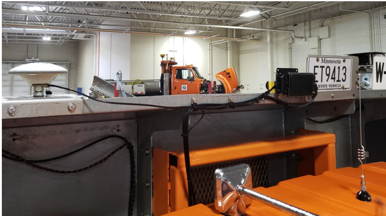
Figure 2.2 GNSS antenna and radar mounted on top of snowplow
