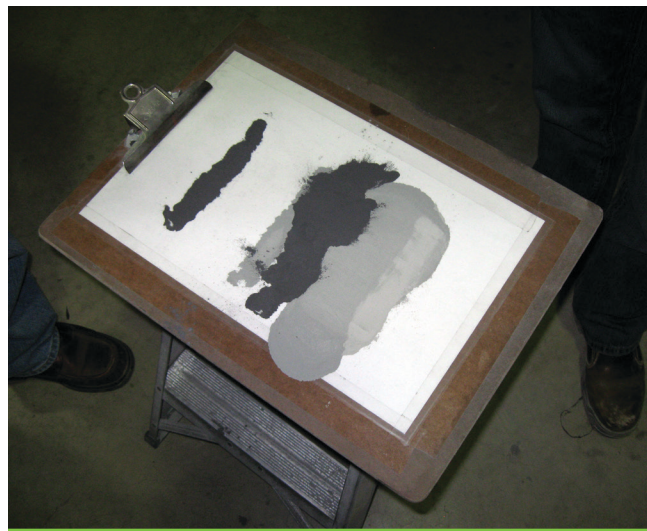
Source: FHWA. A clipboard showing samples of fly ash before and after electrostatic separation to reduce the amount of carbon in fly ash. (7)
