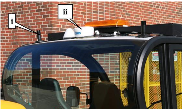
b) Focused Photo of RTK and GPS Antenna
