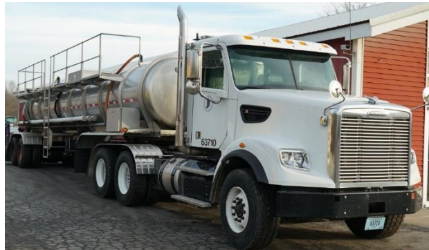
a) Scaling to 5,500-gallon Brine Tanker
