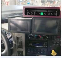
A guidance indicator symbol (green square) from the display unit on the plow dashboard is visible in an operator's peripheral vision.
