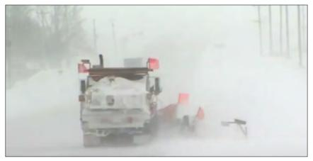
A driver assist system that displays a simple, easy-to-interpret symbol to clearly indicate a warning and provides an audible alert for hazards within the plow's trajectory can significantly enhance safety during whiteout conditions.
