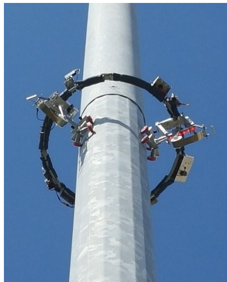
Figure 59. Photo. Remote high mast lighting tower climber.
