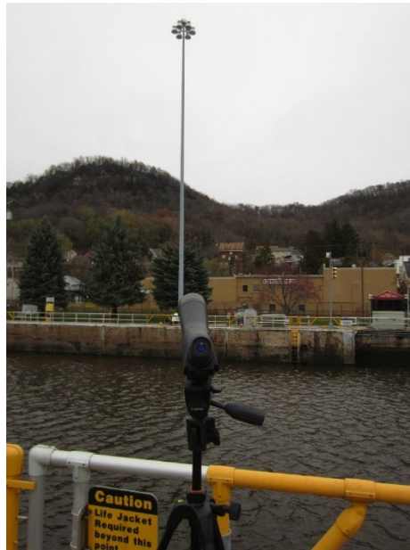
Figure 57. Photo. Spotting scope utilized for viewing the top of a high mast light tower.
