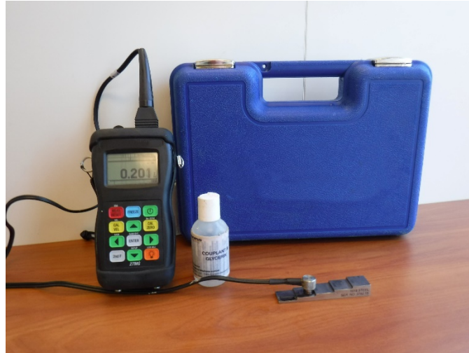
Figure 83. Photo. Typical ultrasonic thickness meter (D-Meter).
