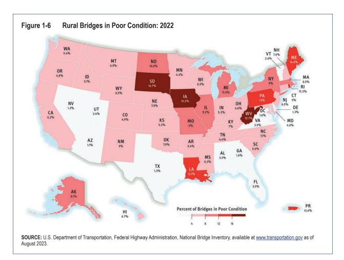
with posted load restrictions are in rural areas. Load restrictions on bridges can increase costs (e.g., delivery delays, costly detours, and the need for lighter trucks or loads). Detours around a closed bridge in rural areas averaged more than three times the distance of bridge detours in urban areas (17.8 versus 5.6 miles) [USDOT OST 2023].
