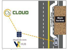
Source: FHWA. V2X Hub = Vehicle-to-Everything Hub.<sup>(5)</sup> Figure 2. Graphic. Road weather management simulation scenario.
