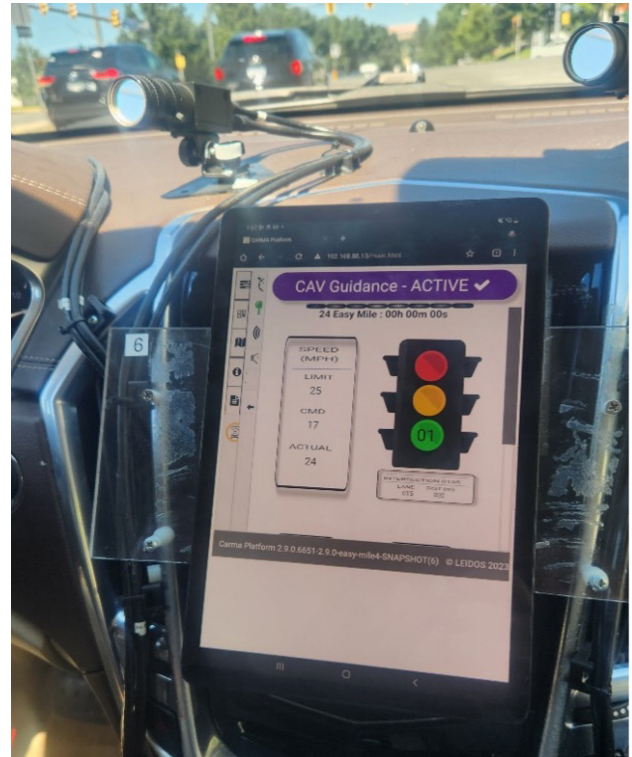
Figure 4. Photo. Comparing intersection crossing behavior of human drivers and AVs below and above 10 mph, data collection featuring the in-vehicle signal phase countdown timer during the dilemma zone.
