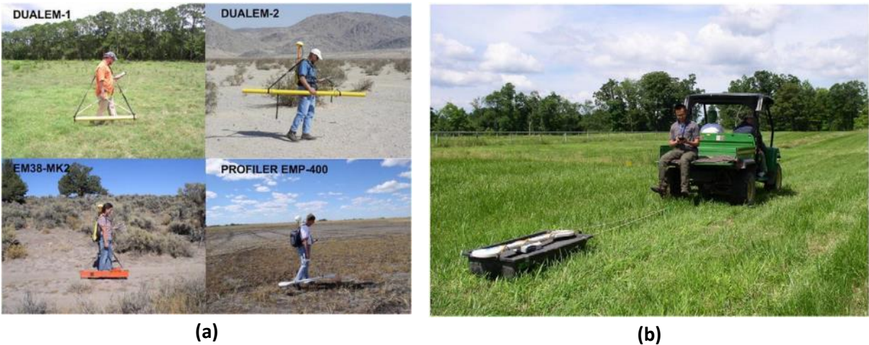
Figure 2.21. Examples of terrain conductivity meters: (a) hand-held units; and (b) mobile towed systems (Corwin 2008).
