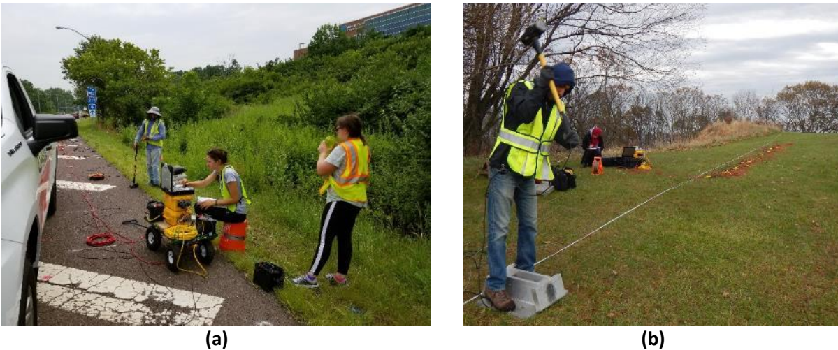
Figure 4.7. Love wave data acquisition: (a) array placed along grassy area next to roadway shoulder; and (b) custom Love wave base plate as used at another site.
