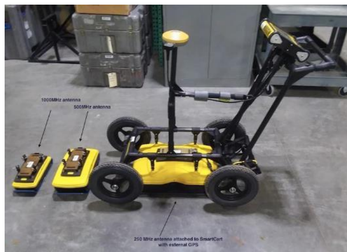
Figure 2.18. GPR systems: (a) schematic/block diagram; and (b) equipment (photo courtesy of IRIS PASSCAL Instrument Center, New Mexico Institute of Mining and Technology https://www.passcal.nmt.edu/ ).
