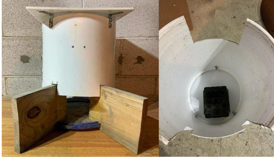
Figure 3. Adapted-Hunt Drift Fence Technique (AHDriFT) camera trap housing unit adapted from Martin et al. (2017). A 5-gallon bucket is inverted with the base removed, and entrance and exit openings cut for animals to pass through. A fixed focal-length camera trap is attached to an acrylic plate, aimed downwards towards the lid. Animals move along the drift fence and are coaxed into the trap and directly under the camera IR sensor by wooden guide boards. The small image frame and short distance of the camera to the lid (about 28 cm) allows for high quality images that can be used to identify small mammal, herpetofauna, bird and invertebrate species.
