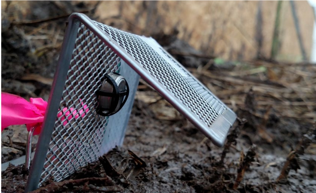
Figure 5. Deployment unit for the Hygrochron iButton Temperature/Humidity Loggers.
