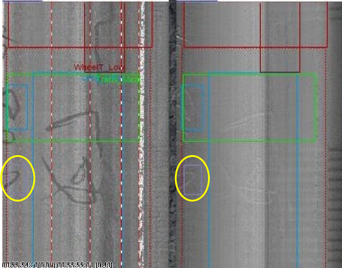
Figure 2.3 Example of an unassigned distress in Pathview, intensity, left and 3D elevation, right
