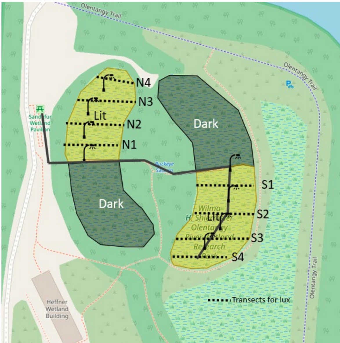
Appendix B Figure 2. Experimental wetland light design at OSU's ORWRP.
