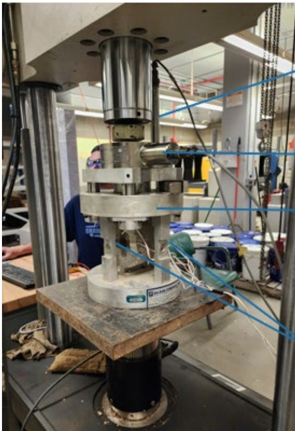
Figure 2. Setup for split tensile test used in second set of tests.
