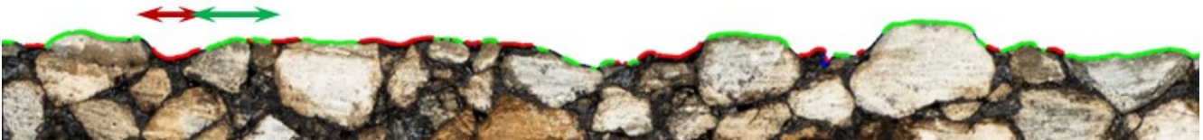
Figure 22. Photo. Side-view image with binder and aggregate separation at the surface.
