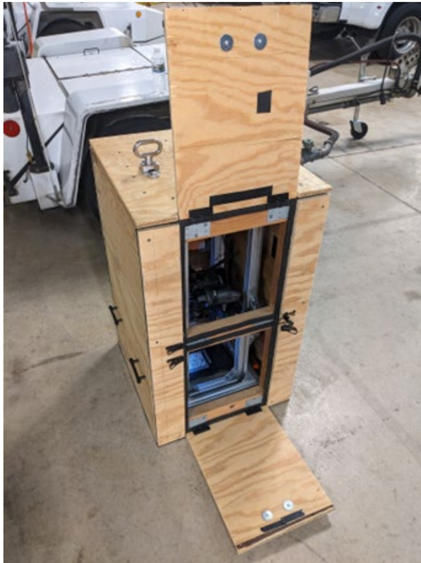
Figure 13. Photo. Overhead scanning-imaging acquisition frame designed and built in this study.
