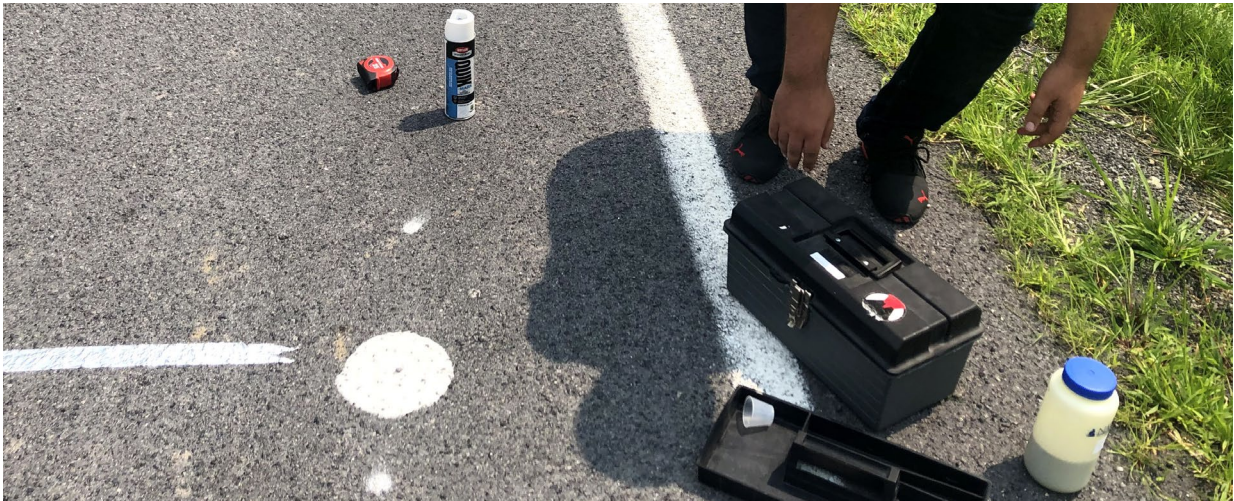
Figure 9. Photo. Sand patch test performed in the field.
