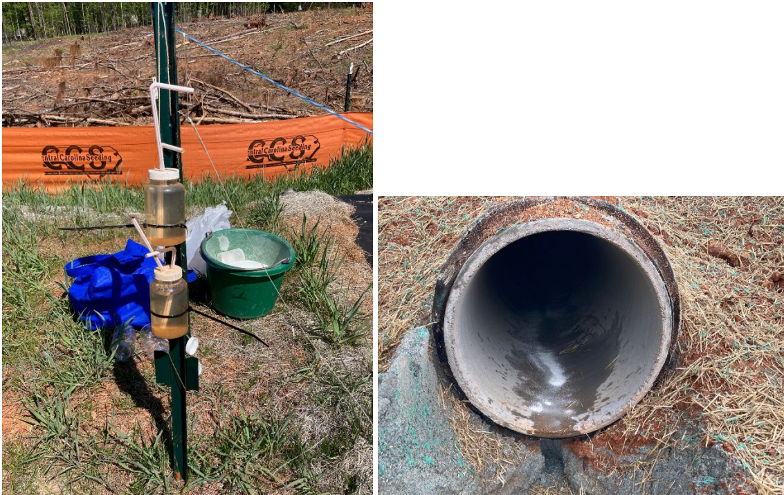
Figure 20. Stage samplers and example of PAM application in storm pipe at the I-40/NC86 site.
