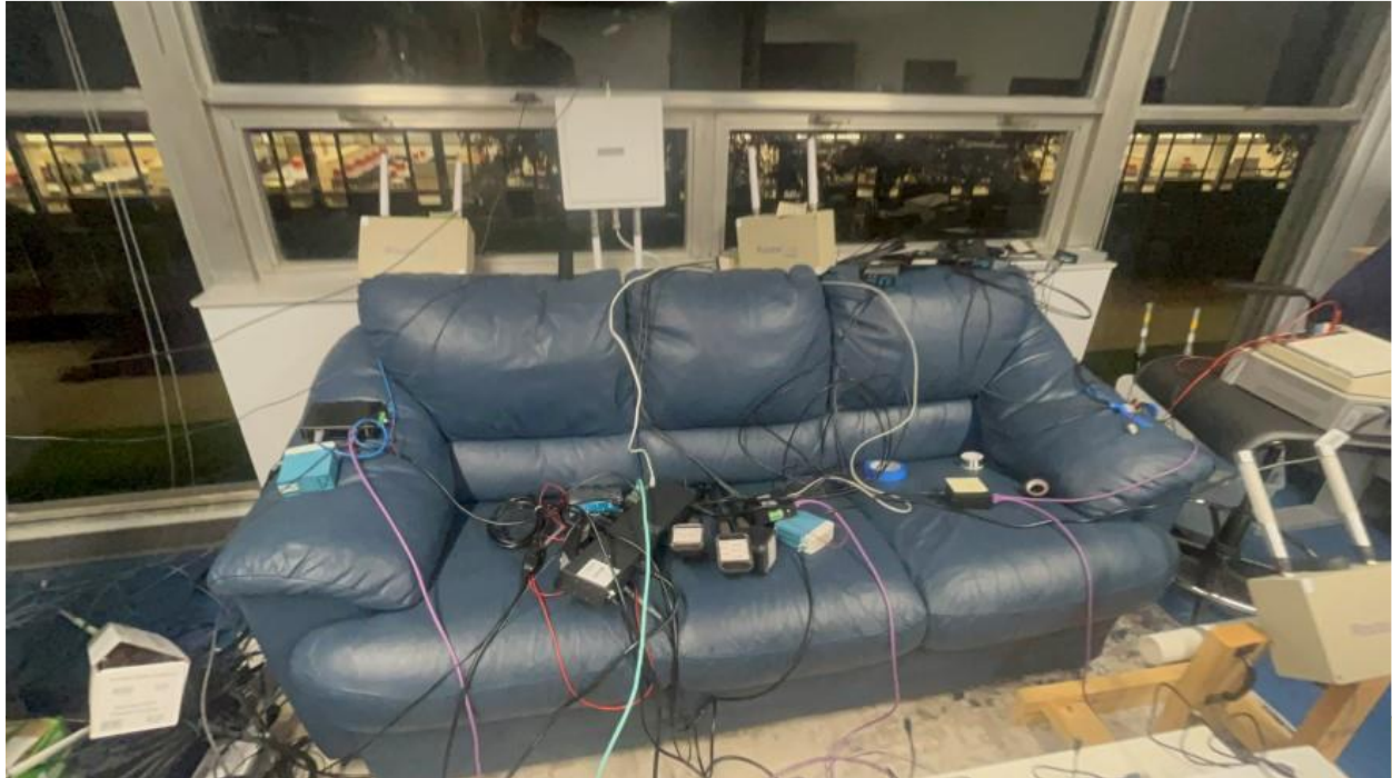
Figure 8. Photo. LTE-V2X 3GPP Rel 14 Sidelink equipment acting as additional interferers at full-rate.
