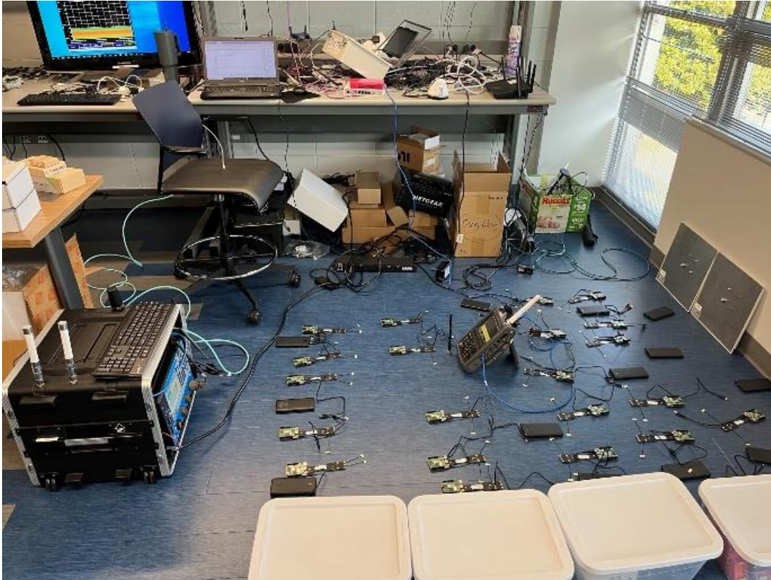
Figure 6. Photo. Test set-up for DSRC U-NII-4 interference tests.
