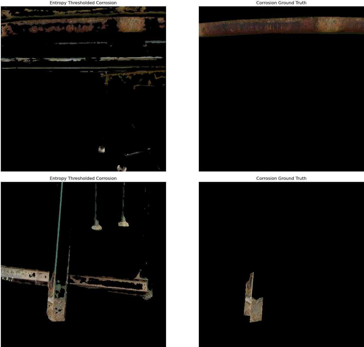
Figure 15. Photographs. Results of entropy thresholding on images with background removed using the labels.
