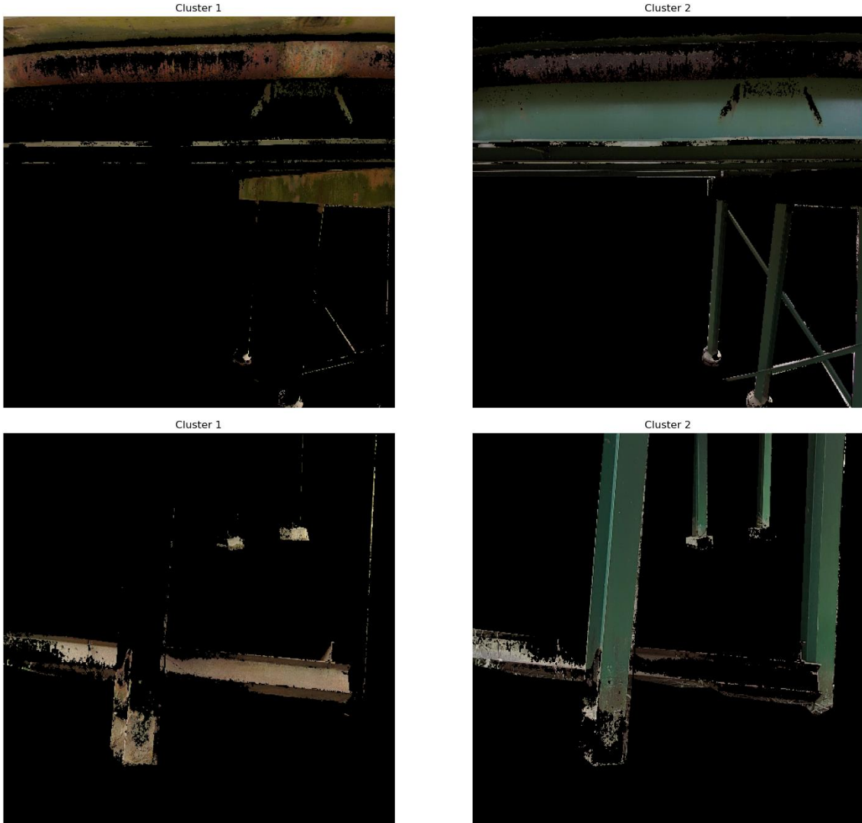
Figure 20. Photographs. Results of color thresholding on images with background removed using the ground truth.
