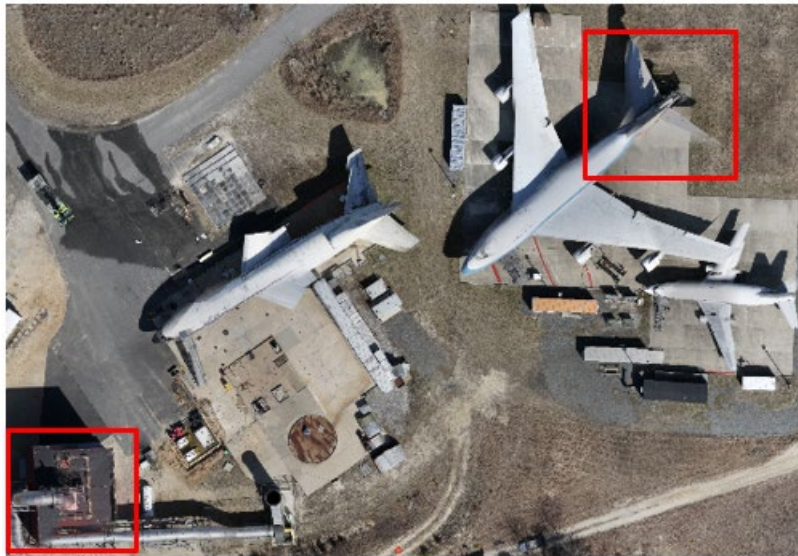
Figure 25. Errors in 0.5-in. GSD WingtraOne Data Set Processed with Pix4DReact
