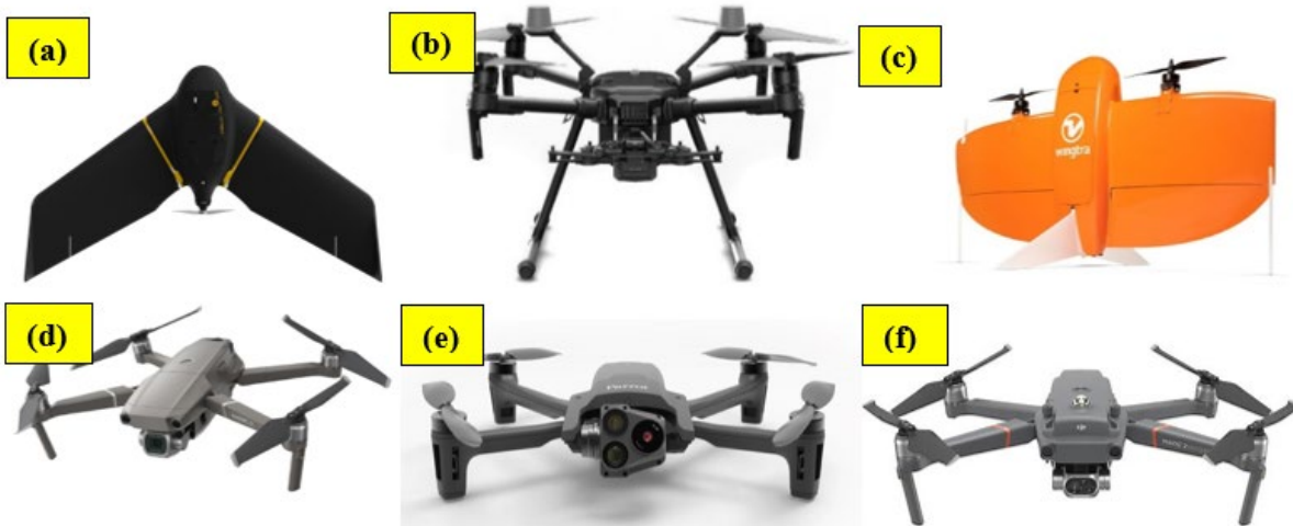
Figure 6. UAS Platforms: (a) eBee X, (b) M210, (c) WingtraOne, (d) Mavic 2 Pro, (e) Parrot ANAFI USA, and (f) M2ED
