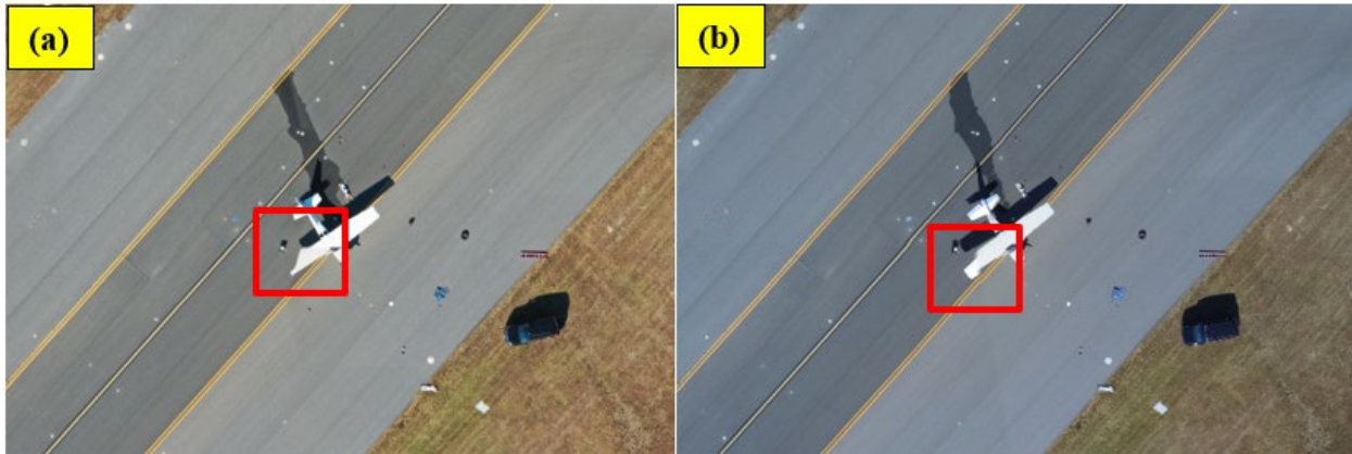
Figure 36. C172 Wingtip Distortion in Pix4DReact Orthomosaics from (a) Test 1A (70%/60% overlap and 0.39-in. GSD) and (b) Test 3 (70%/60% overlap and 1-in. GSD)
