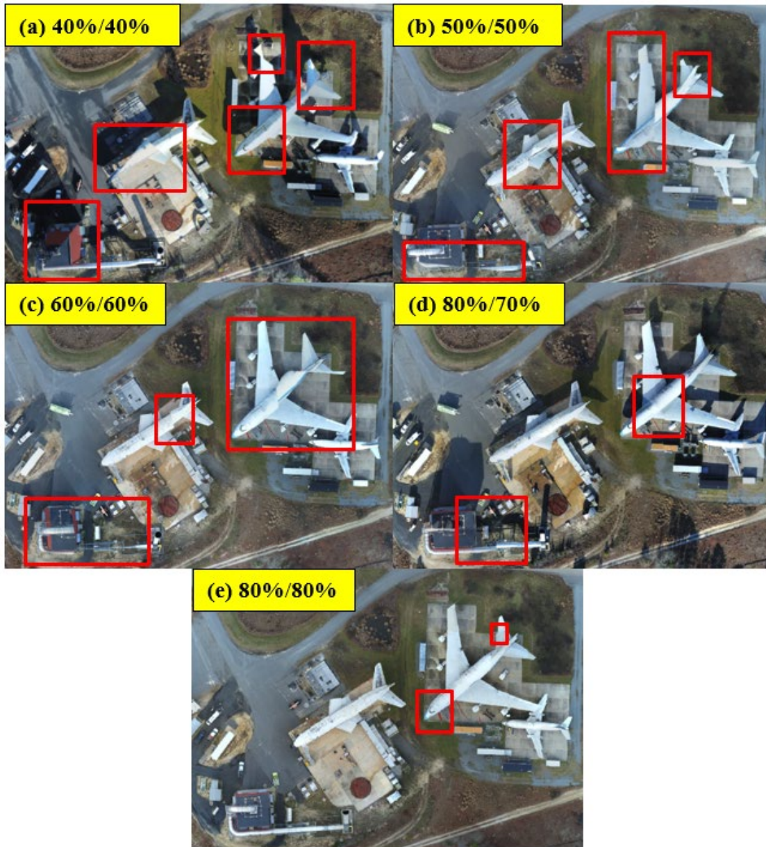
Figure 48. Comparison of Distortion Present in Data Sets Collected with Various Overlap Settings with the ANAFI USA and Processed with Pix4DReact
