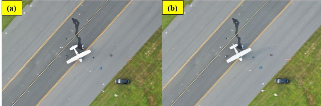
Figure 38. Comparison of Distortion in Orthomosaics Generated by Pix4DReact from Data Sets Collected by the Mavic 2 Pro with Overlap Settings of (a) 80%/70% and (b) 40%/40%
