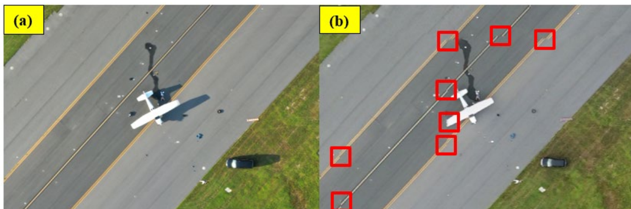
Figure 37. Comparison of Distortion in Orthomosaics Generated from Test 6 (60%/60% overlap and 1-in. GSD) by (a) Pix4DReact and (b) DroneDeploy LiveMap
