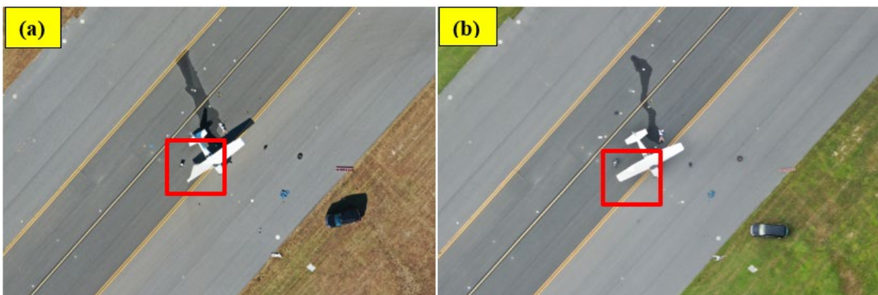
Figure 39. C172 Wingtip Distortion in Pix4DReact Orthomosaics from (a) Test 1A (70%/60% overlap and 0.39-in. GSD) and (b) Test 5A (70%/60% overlap and 1-in. GSD)
