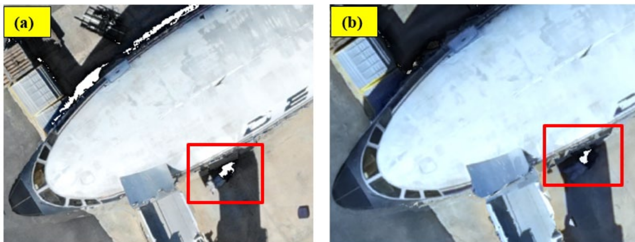
Figure 22. White Clipping Obscuring Manikin in 1-in. GSD Data Sets Processed with Maps Made Easy and Collected with the (a) M2ED and (b) Parrot ANAFI USA
