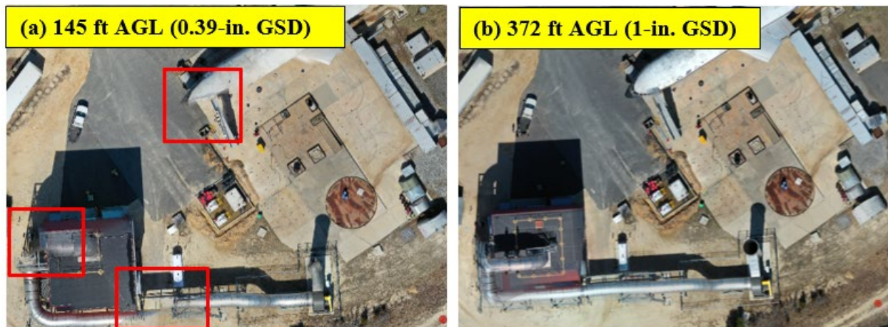
Figure 26. Comparison of Distortion in Mavic 2 Pro Data Sets Processed with Pix4DReact and Captured at (a) 145 ft AGL and (b) 372 ft AGL
