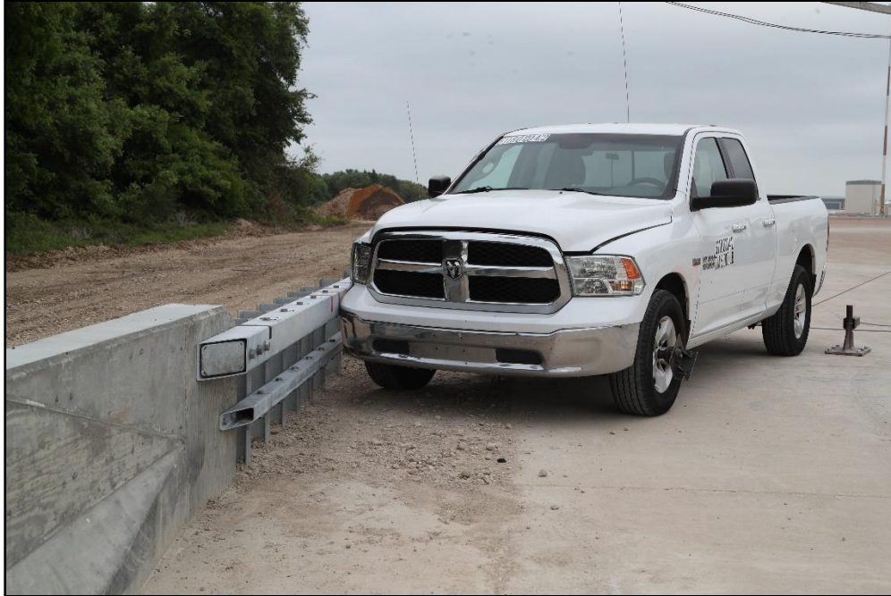
Figure 7.17. Box Beam to Concrete Barrier Transition/Test Vehicle Geometrics for Test 611801-04-2.
