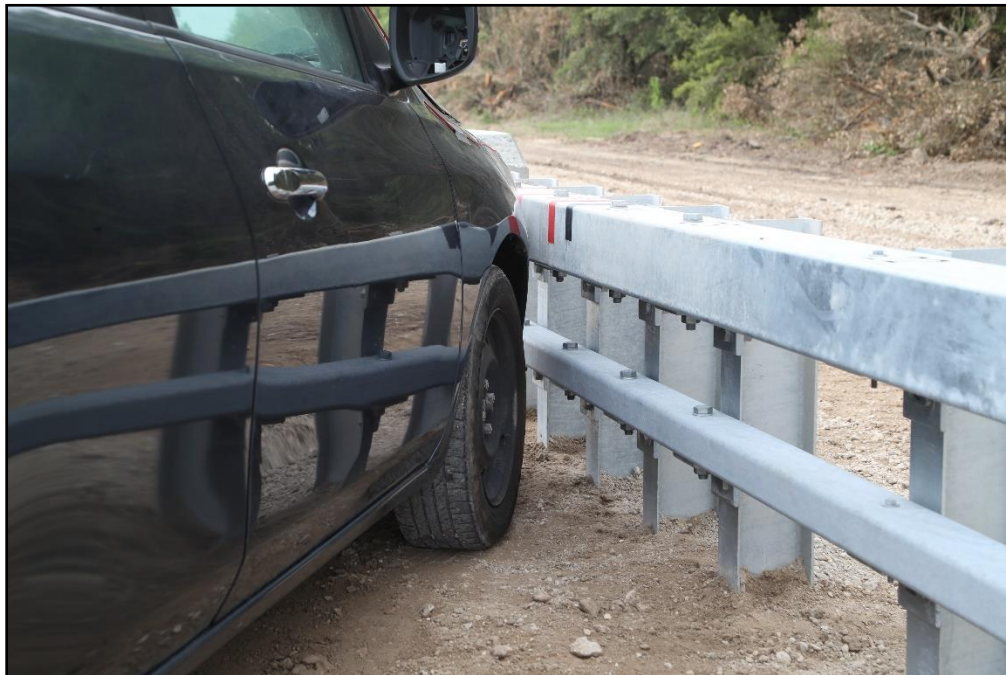
Figure 7.7. Box Beam to Concrete Barrier Transition/Test Vehicle Impact Location 611801-04-1.
