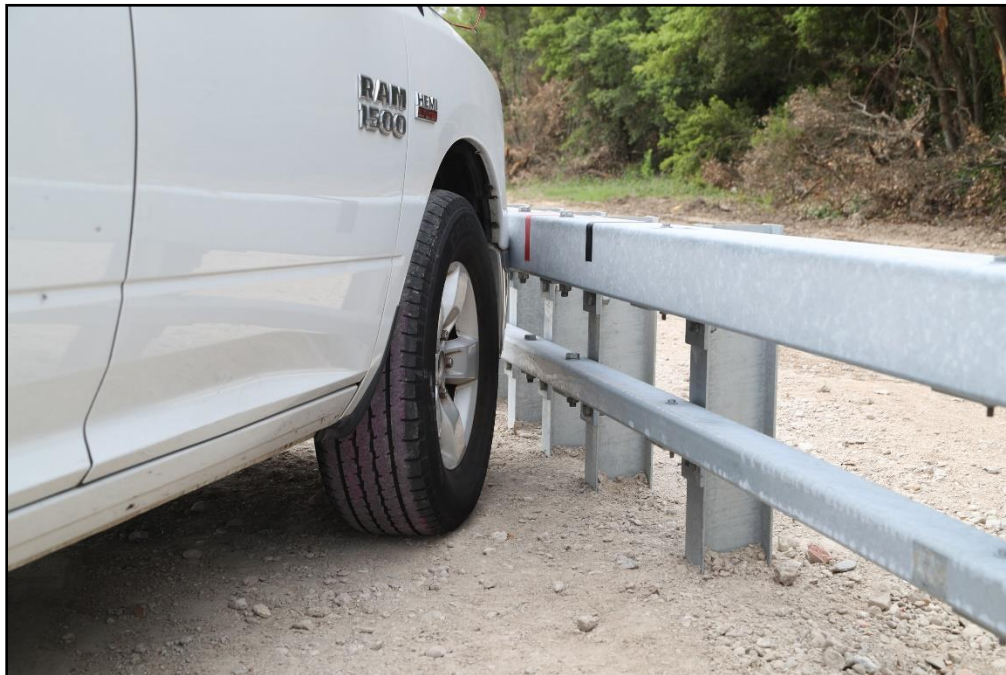
Figure 7.18. Box Beam to Concrete Barrier Transition/Test Vehicle Impact Location 611801-04-2.
