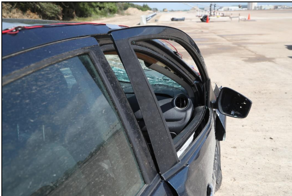
Figure 7.13. Door on the Impact Side of Test Vehicle after Test 611801-04-1.
