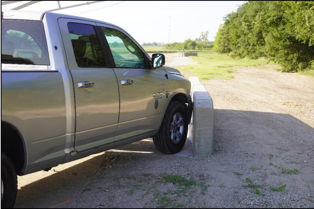
Figure 6.18. Concrete Parapet Shape Transition/Test Vehicle Impact Location 611801-03-2.
