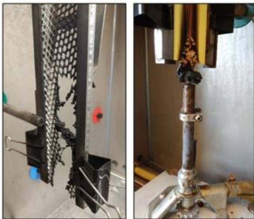
Figure 11. Sample melted away (left) and melted material blocking Bunsen burner flame (right)
