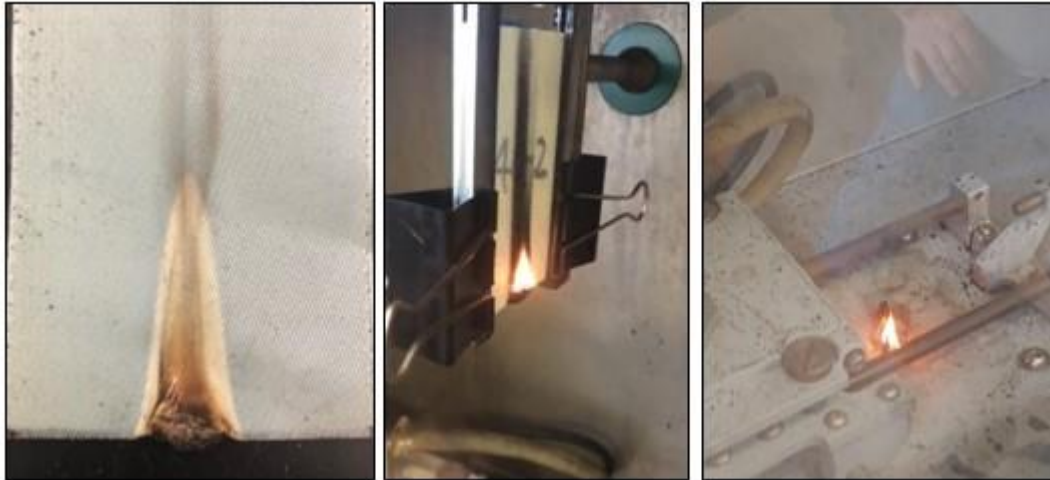
Figure 6. Burn Length, flame time, and drip flame time measurements, respectively
