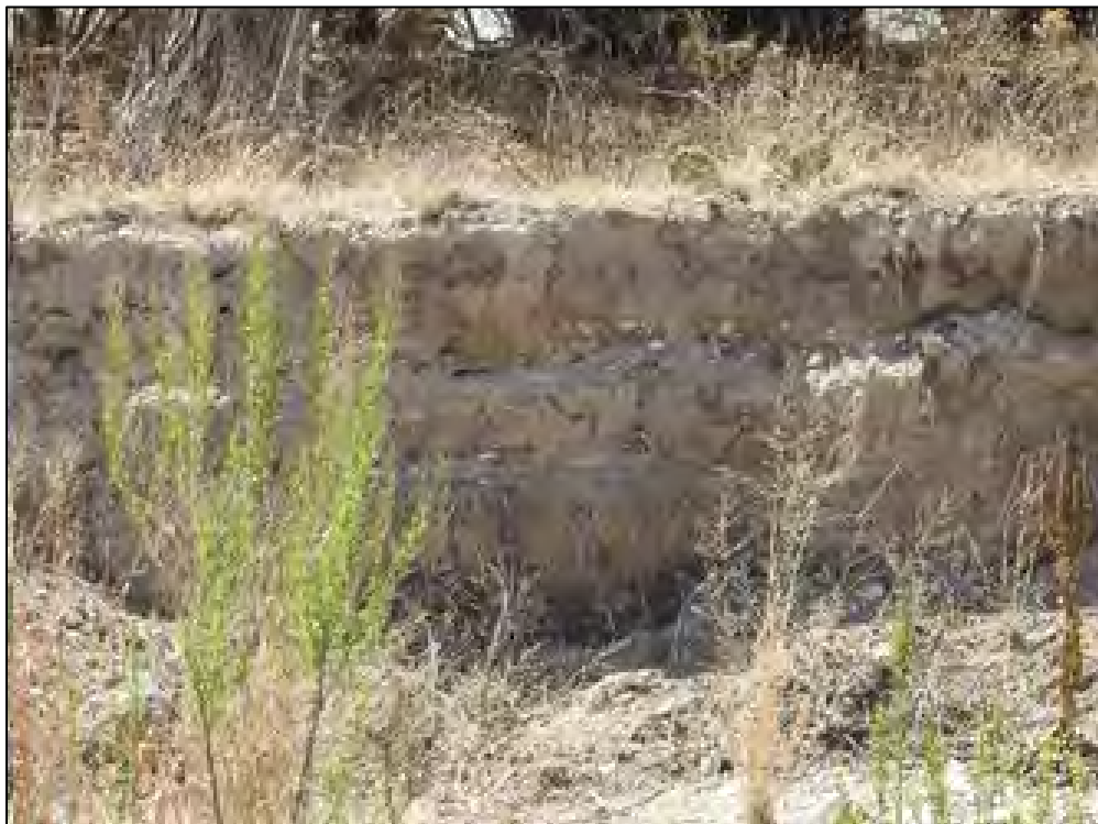
Figure 7.20. Potential PSI in a flood deposit: interspersed coarse and fine sediment layers indicating different flood deposits. Source: Desert Sky Engineering and Hydrology and used by permission.
