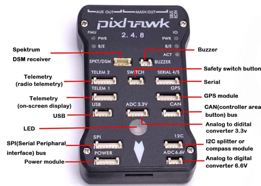
Figure 6. PXI PX4 Pixhawk 2.4.8 Flight Controller
