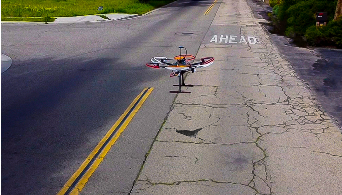
Figure 29. Experiments Conducted to Detect Faults in the Road Using the Prototype Quadcopter Drone
