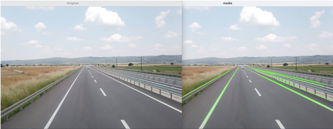
Figure 26. Hough Transform Performed on a Roadway Image: Original and Modified
