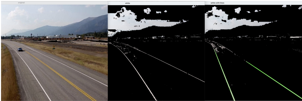
Figure 27. Color Masking and Hough Transform Performed on a Roadway Image
