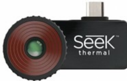
Figure 10. Seek Thermal CompactPRO Infrared Camera
