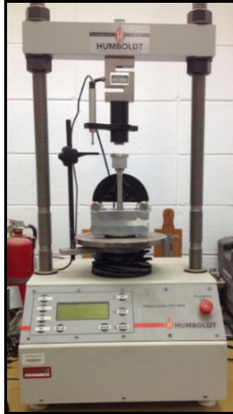
Figure 2 Semi-circular bending device
