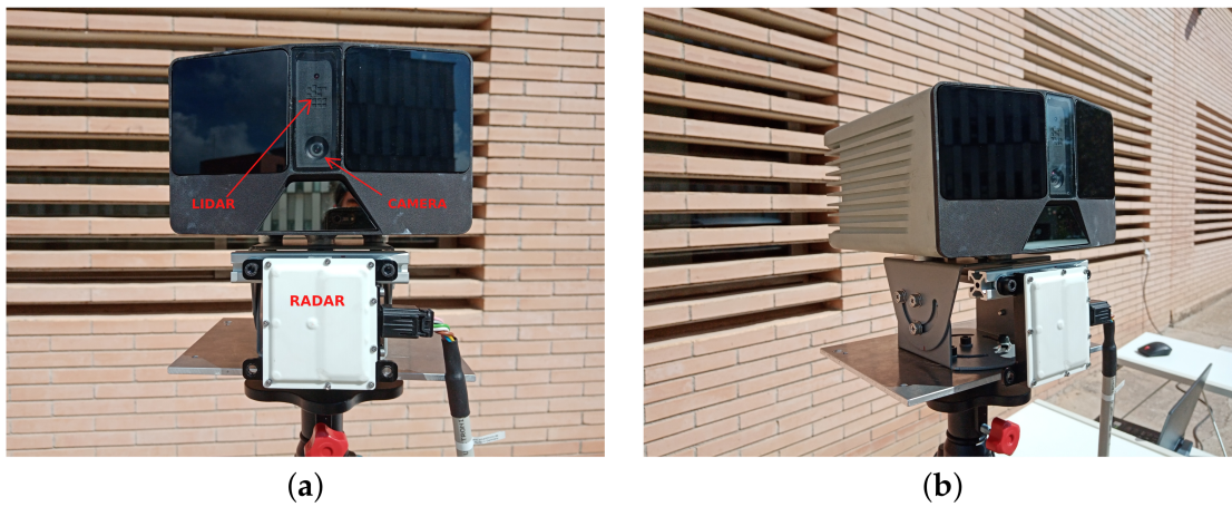
Figure 10: Example of a setup for Multi-Sensor Fusion [305]
