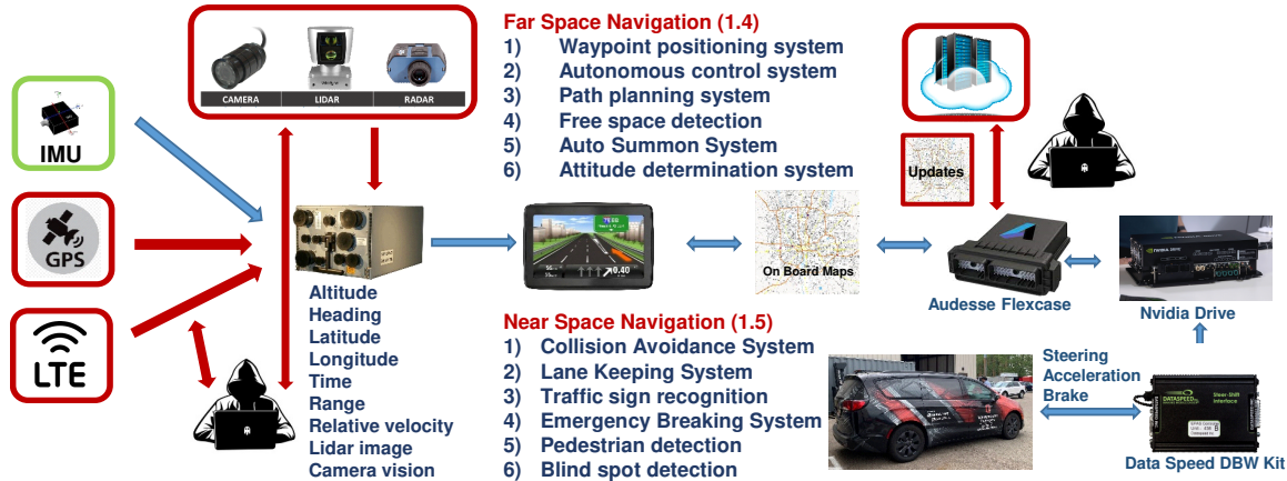
Figure 11: Framework for onboard subsystems and sensors for far-space and near space navigation
