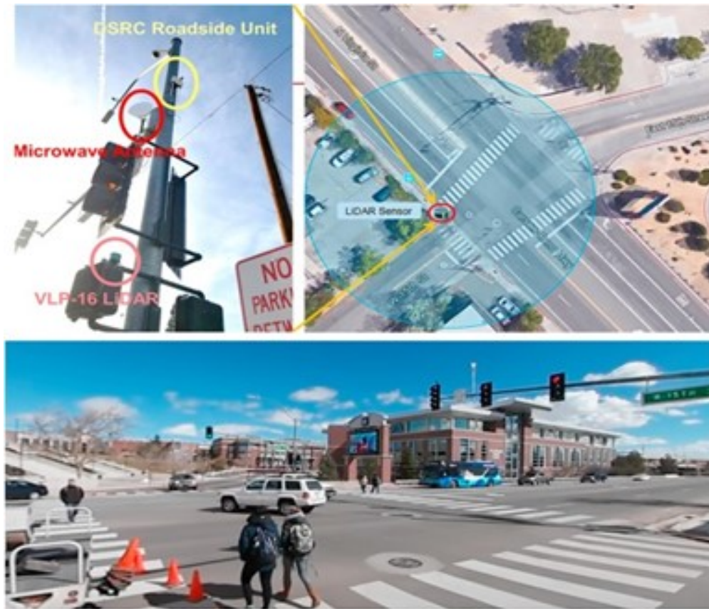
Figure 9: Infrastructure-based LiDAR implementation by Nevada DOT [302]
