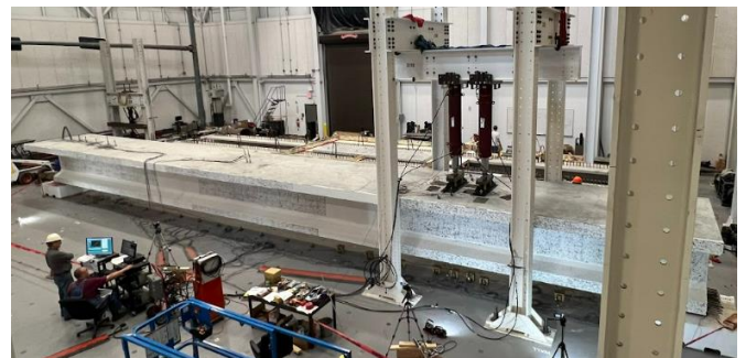
Figure 1. Testing of Full-Scale Girder with Conventional Concrete Deck.
