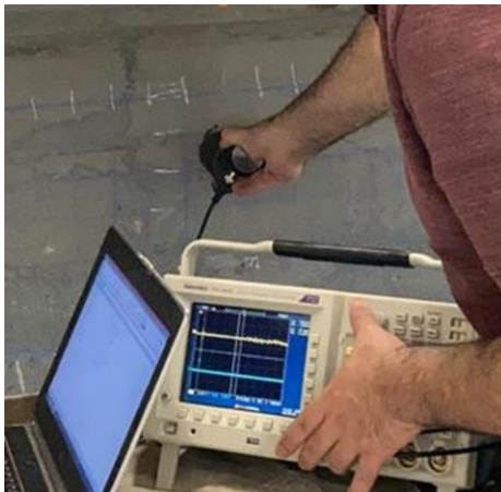
(c) UPV in Progress
