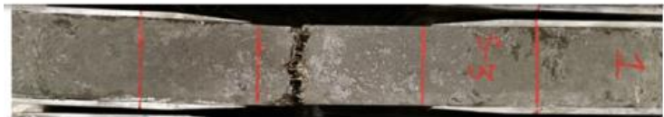
(c) Specimen 03 cracked within the gage length
