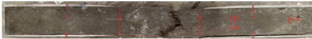
(a) Crack occurring within the gage length
