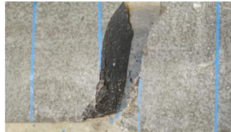
(c) As-cast specimen 05: Side face – fibers settled at bottom with no fibers at top
