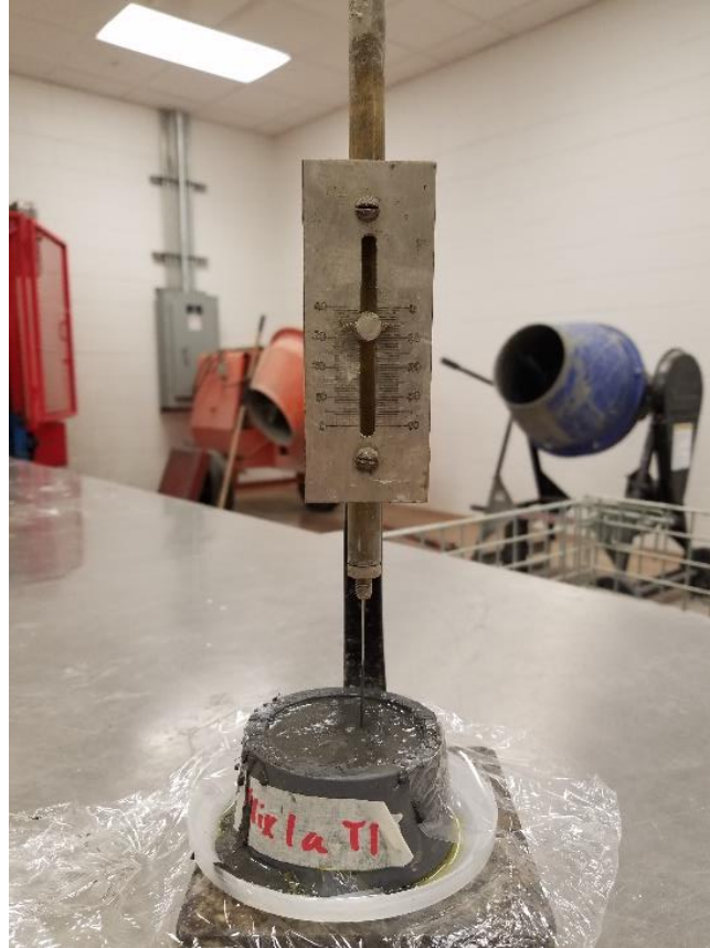
Figure 3.2. Time of Setting in Accordance with Modified ASTM C191 (2018).
