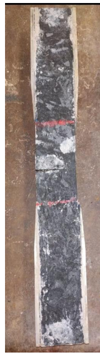
(b) Specimen after being tested—crack within gage length
