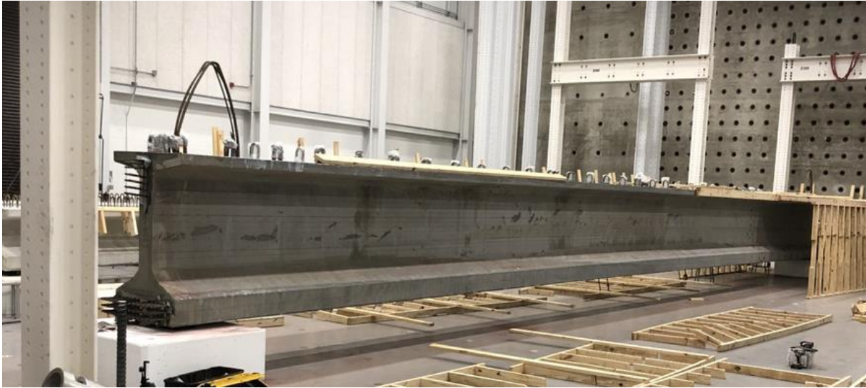
Figure 7.6. Tx54 after Completion of Thermal Imaging Recording.
