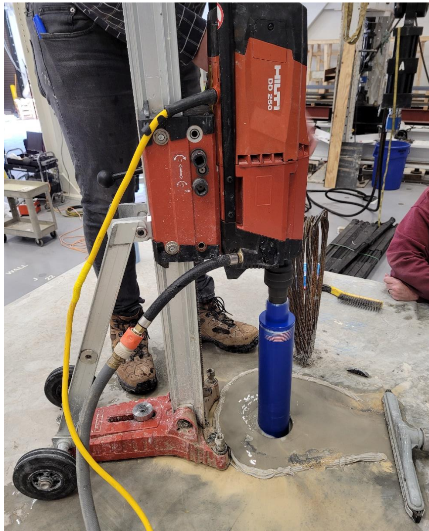
Figure 8.1. Coring UHPC Girder Using Hilti DD-250 Coring Machine.
