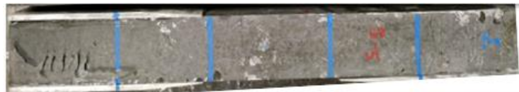
(e) Specimen 05 cracked within the grips
