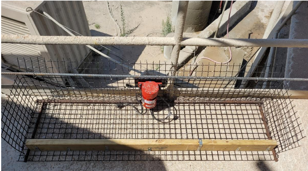
Figure 6.1. Fabricated Vibrator-Equipped Screen for Steel Fiber Addition.
