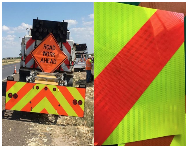
Figure 26. The Location of Chevron Stripes on the Vehicles (TDOT, 2018).
