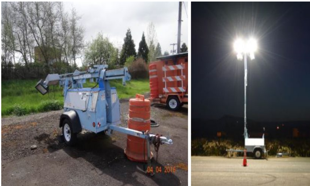
Figure 37. Portable Trailer-Mounted Light Tower with Mast Lowered and Mast Raised (Gambatese, J., And Jafarnejad, A.,2018).
