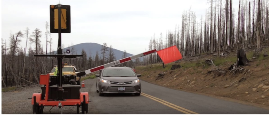
Figure 47. Oregon DOT Using New Auto Flagging Technology to Protect Road Workers (Roads & Bridges, 2019).
