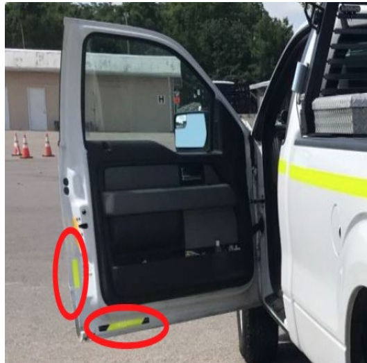
Figure 25. Tape On the Inside Door to Face Traffic When Door is Opened (TDOT, 2018).
