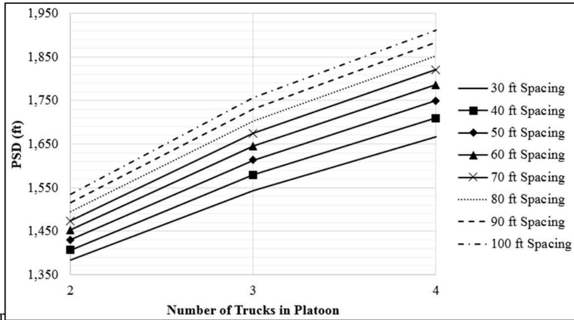
Figure 19: Computed passing sight distances for overtaking oil and gas truck platoons on a 70-mph two-lane highway.
