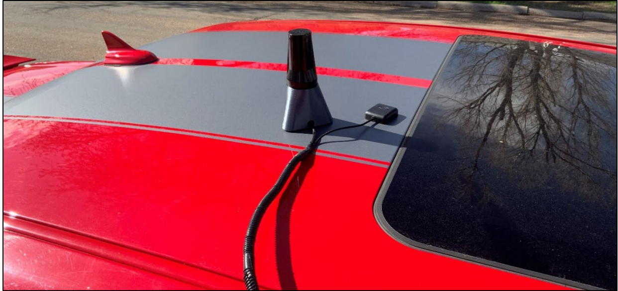
Step 4: Attach the antennas to the roof of the vehicle.
