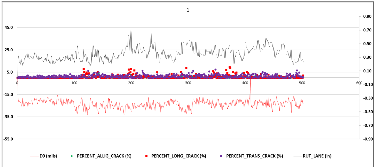
Figure 10.16 SH-26 TSD Deflection (D0) Vs. Pavement Distresses
