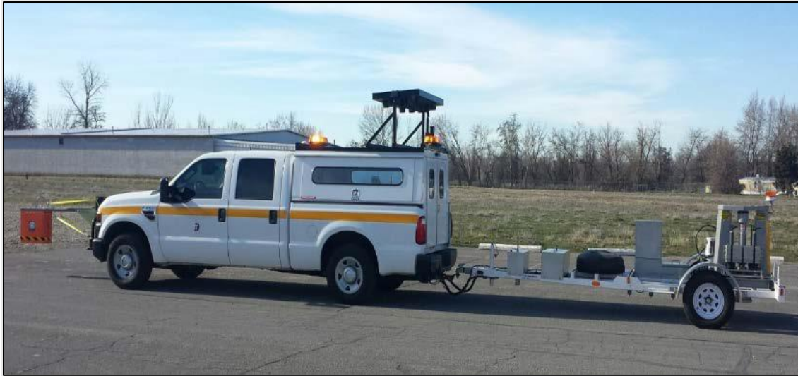
Figure 2.2 Current FWD used by Idaho Transportation Department (ITD) with Truck and GPS horn (ITD 2017)
