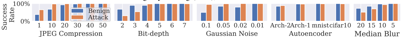
Fig. 35: Evaluation results for 5 directly-applicable DNN model level defense methods. Attack : Attack success rate. Benign : Percentage of scenarios where the ALC can still behave correctly (i.e., not driving out of current lane) with defense applied.
