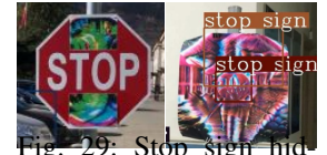
Fig. 29: Stop sign hiding and appearing attacks [154].
