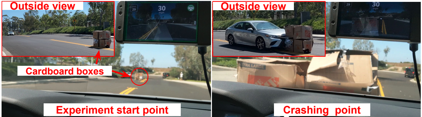
Fig. 34: Safety impact evaluation for our attack on a Toyota 2019 Camry with OpenPilot engaged. Even with other driver assistance features such as Automatic Emergency Braking (AEB), our attack still causes collisions in all the 10 trials.
