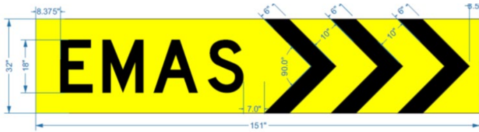
Figure 5. Conceptual EMAS Sign Dimensions
