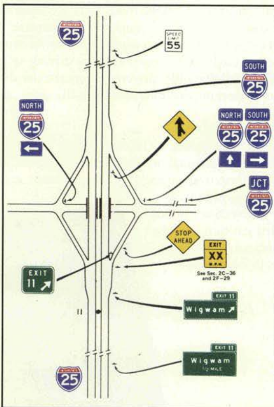
The MUTCD provides detailed recommendations on how to properly "sign" an interstate intersection (left) or provide safe directions for a motorist passing through a work zone (right).
