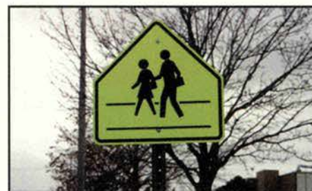
The new fluorescent yellow green warning signs are officially recommended for use by FHWA.
