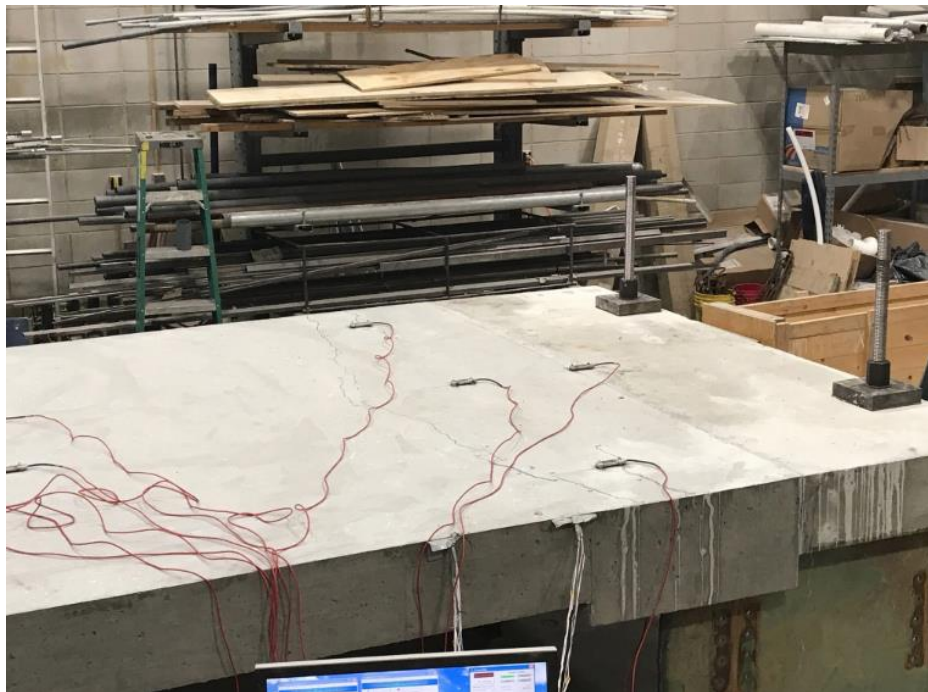
Figure 4.7. BDI on laboratory specimen
