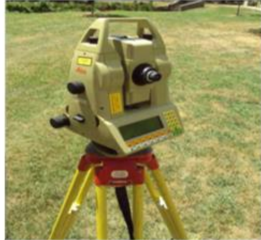
Figure 6.1. Surveying prism (left), total station (right)
