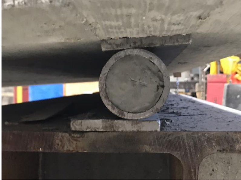
Figure 4.34. Horizontal movement of the slab at the roller support, Test 2
