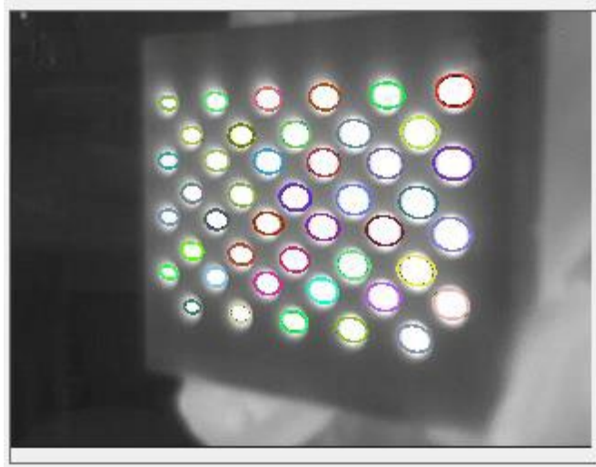
Figure 6. Thermal image of the symmetrical circular pattern.
