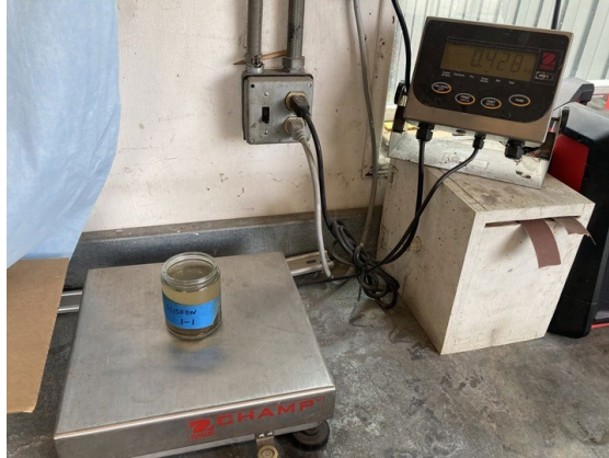
Figure 15. Photo. Water/sediment sample weighing (W1).
