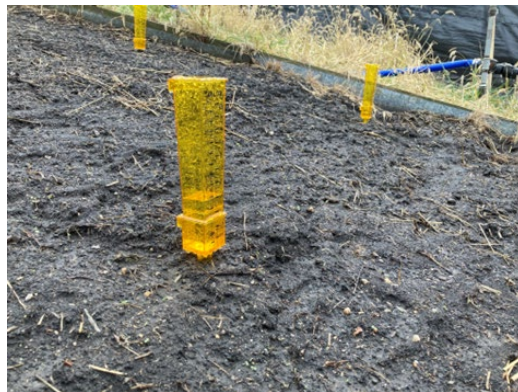
A. Rain gauge mounted on the slope
