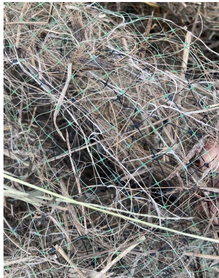
Figure 40. Photo. Plastic net left on-site permanently.
