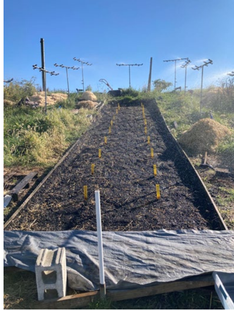
Figure 9. Photo. Test plot with rain gauges and tarp on the pan avoiding direct rainfall.
