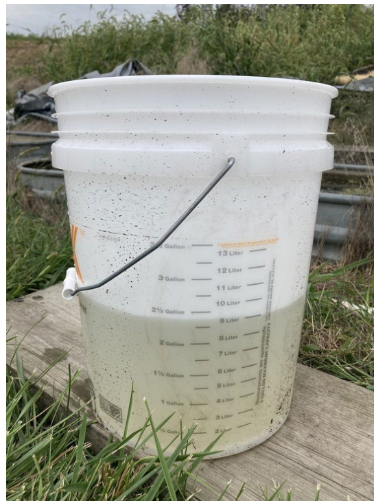
Figure 14. Photo. Runoff reading (13-liter capacity).
