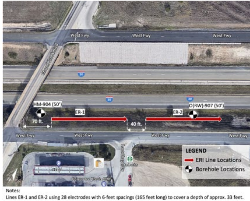
Figure 4.14. ERI data collection plan and borehole locations for IH 30 at Chapel Creek Blvd
