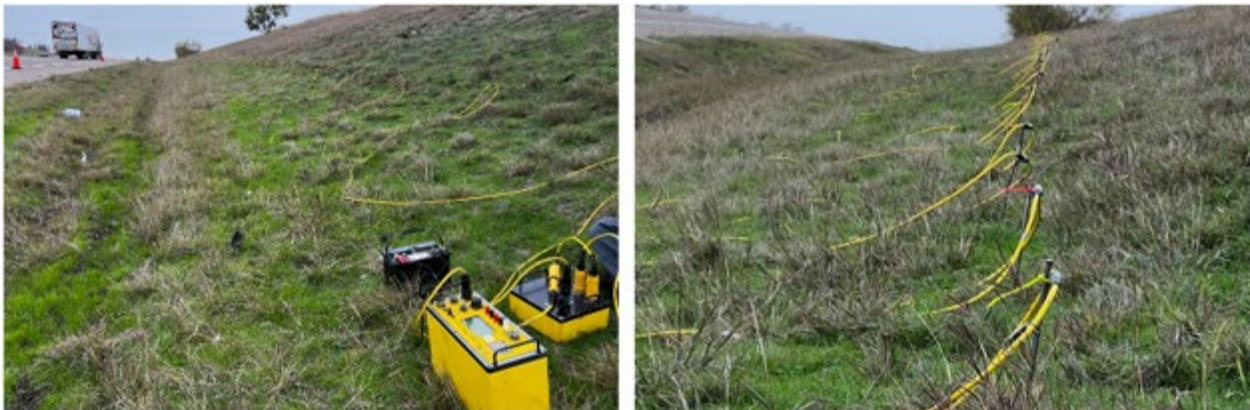
Figure 4.7. Implementation of the ERI along Ronald Reagan Memorial Hwy
