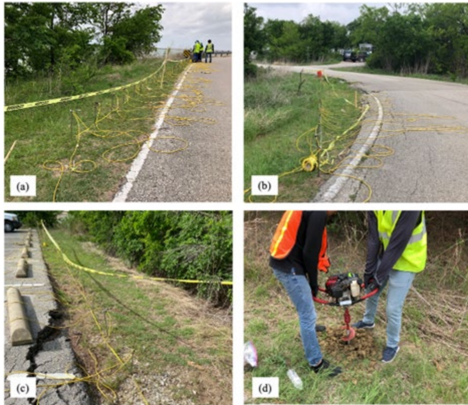
Figure 2.17. Implementation of ERI for Cedar Hill State Park; (a) Line 1 in Zone 1, (b) Line 2 in Zone 2, (c) Line 2 in Zone 2, and (d) soil sampling.
