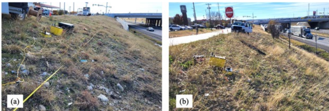
Figure 2.39. Implementation of the ERI along IH 30 at Chapel Creek Blvd; (a) Line ER-1 and (b) Line ER-2
