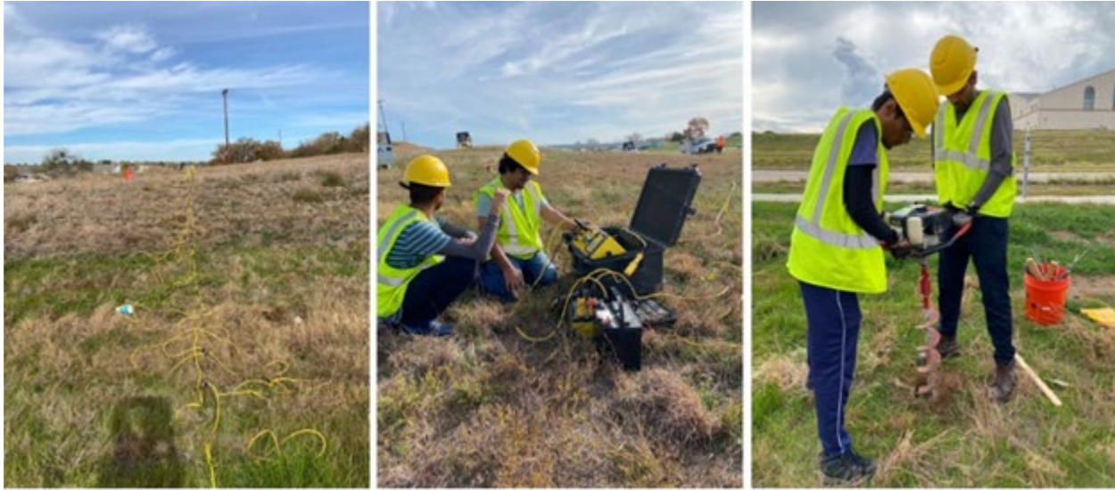
Figure 2.3. Implementation of ERI along highway US 67 and soil sample collection
