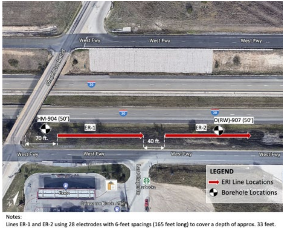
Figure 2.38. ERI data collection plan and borehole locations for IH 30 at Chapel Creek Blvd In coordination with the Fort Worth district contacts, the research team implemented the ERI plan for IH 30 at Chapel Creek Blvd on December 2 nd , 2022. Two ERI surveys were conducted using 28 electrodes with 2 feet spacings. Figure 2.39 shows the implementation of the ERI along IH 30 at Chapel Creek Blvd. In a week before the implementation, 0.49 inches of precipitation were recorded at the site (Weather Underground 2022).
