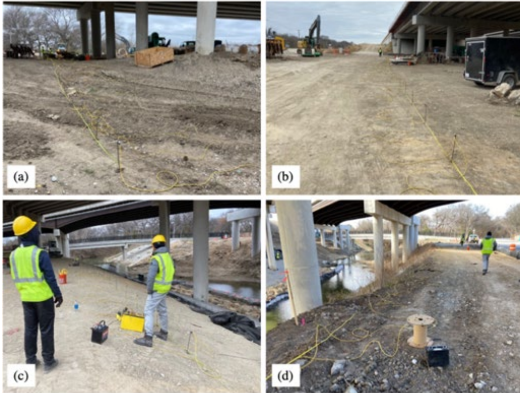
Figure 2.12. Implementation of ERI for IH 20 project; (a) on the crest of the slope at the river's West bank, (b) on the crest of the slope perpendicular to the river, (c) on the middle of the slope on the river's West bank, and (d) on the crest of the slope on the river's East bank.
