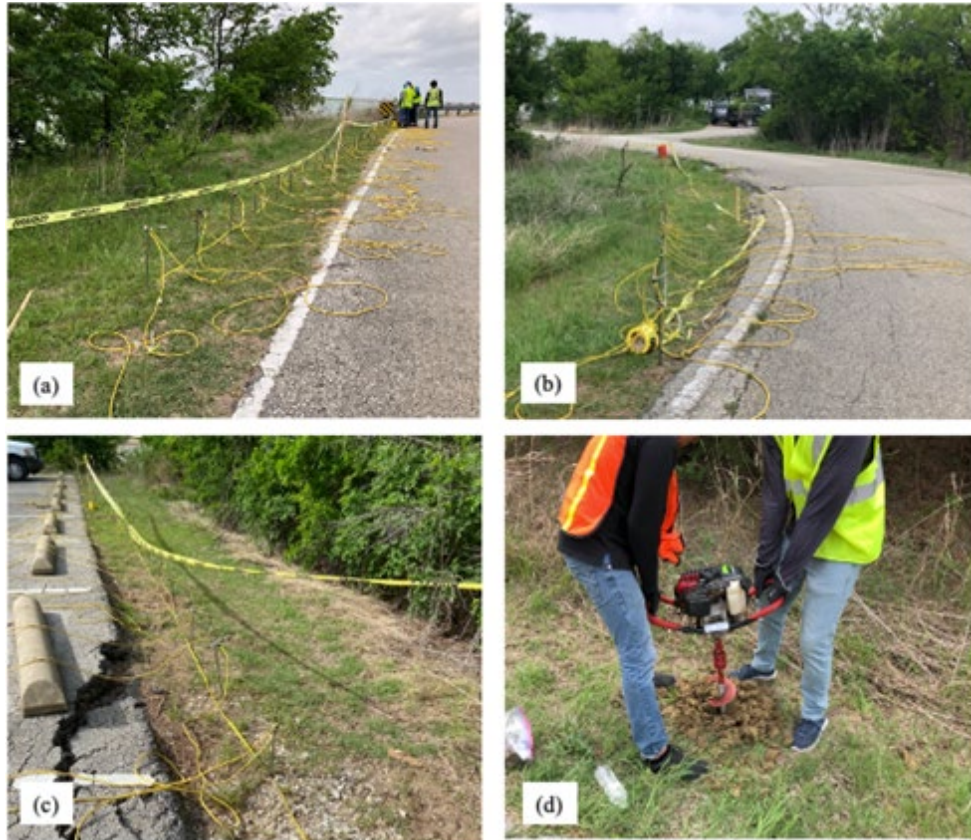
Figure 4.2. Implementation of ERI for Cedar Hill State Park; (a) Line 1 in Zone 1, (b) Line 2 in Zone 2, (c) Line 2 in Zone 2, and (d) soil sampling.
