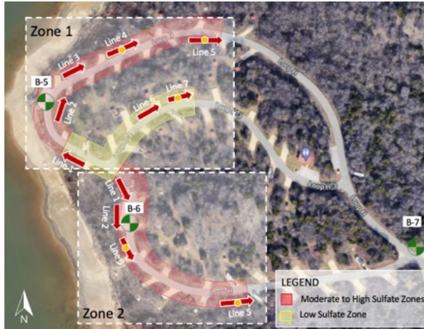
Figure 2.21. Overview of the extent of critical zones with the risk of sulfate-induced heaving
