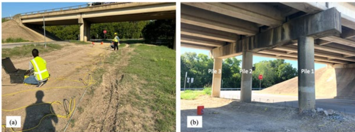
Figure 2.34. Implementation of the ERI along Mary's Creek; (a) ER-1 and (b) ER-2 within a small distance from the bridge piles
