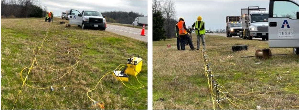
Figure 2.60. Implementation of the ERI along Ronald Reagan Memorial Hwy and soil sample collection
