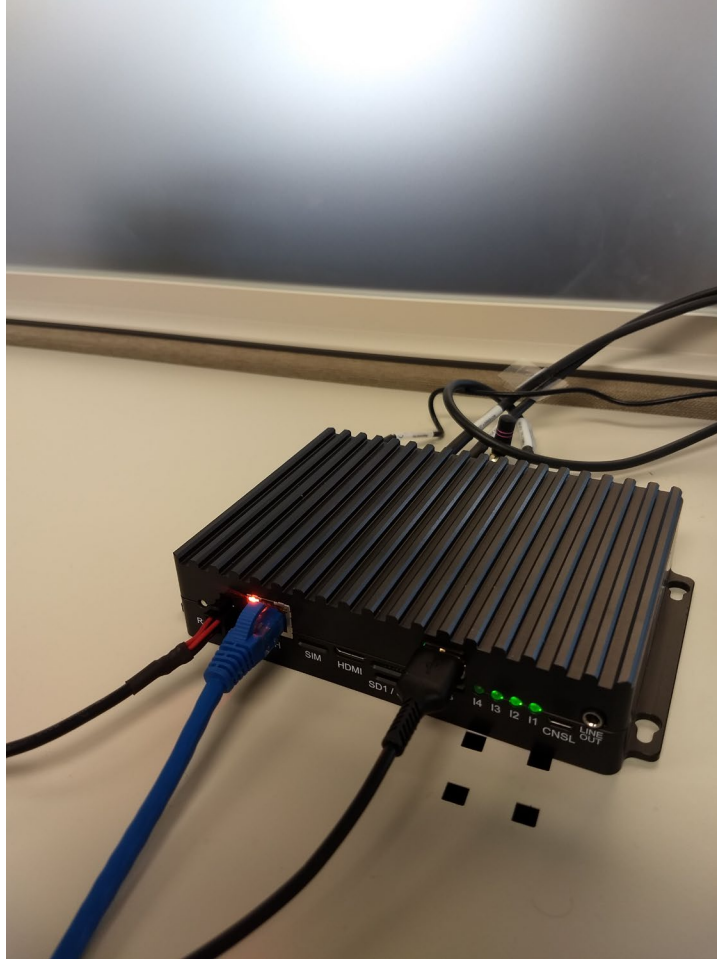
Figure 3-34. Commsignia OBU. Source: WYDOT
