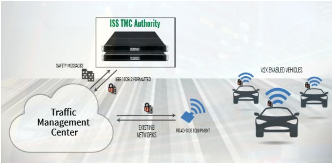
Figure 3-10. HSM working diagram. Source: Integrated Security Solutions
