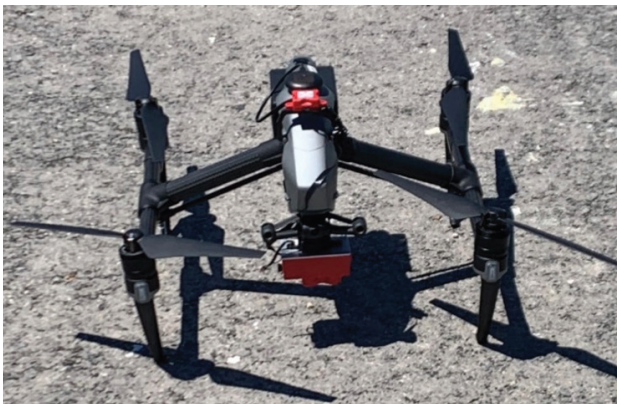
Figure 2. MicaSense RedEdge multispectral camera mounted on DJI Inspire 2
