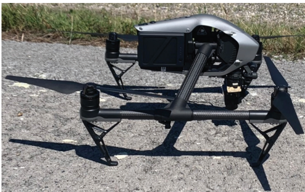
Figure 1. FLIR Vue Pro R thermal camera mounted on DJI Inspire 2
