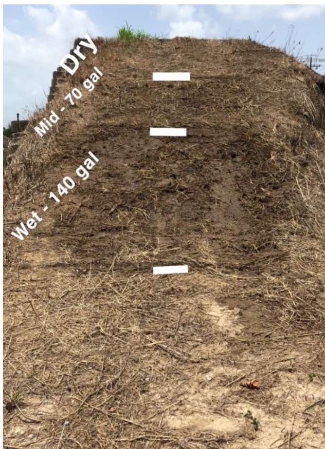
Figure 31. Embankment soil with different moisture contents during flight session 3
