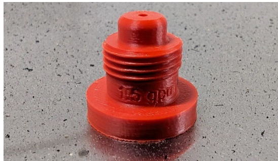
Figure 9. A 3D-Printed, 1.5-gpm Orifice for Mil-Spec Nozzle
