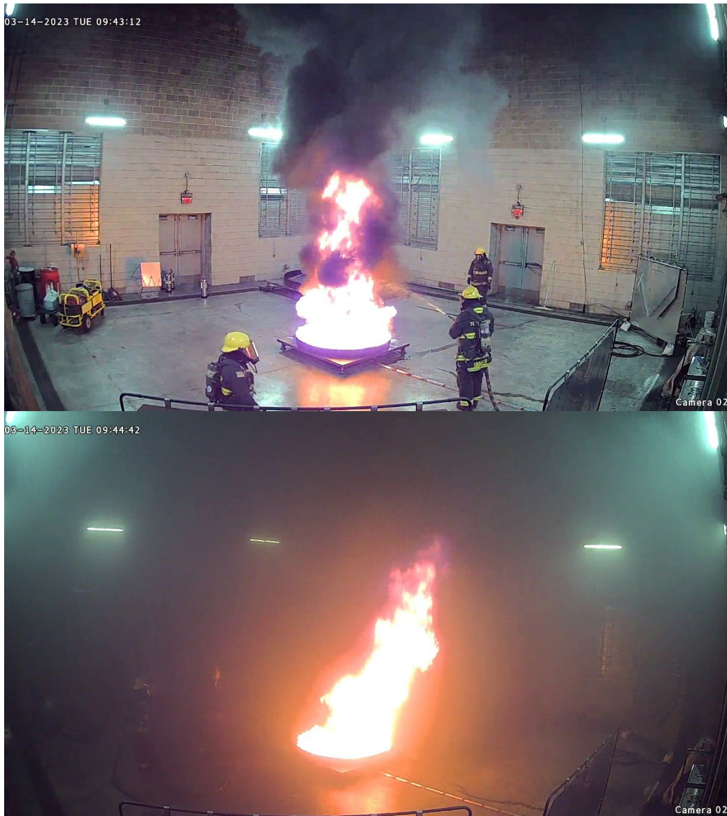
Figure 22. Fire at Beginning (Top) and End (Bottom) of Discharge in Mixed Short-Term Stability with National Foam Avio F3 Green KHC and Solberg Avigard
