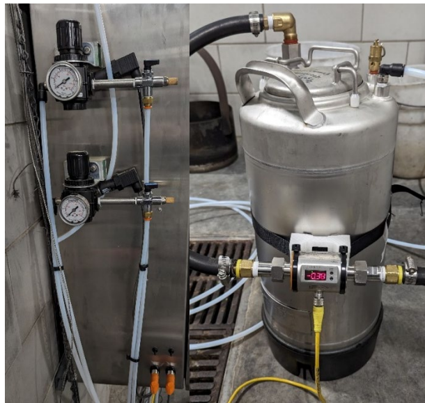
Figure 7. Pressure Control (Left) and Small Extinguisher (Right) for Dual Extinguisher Tests
